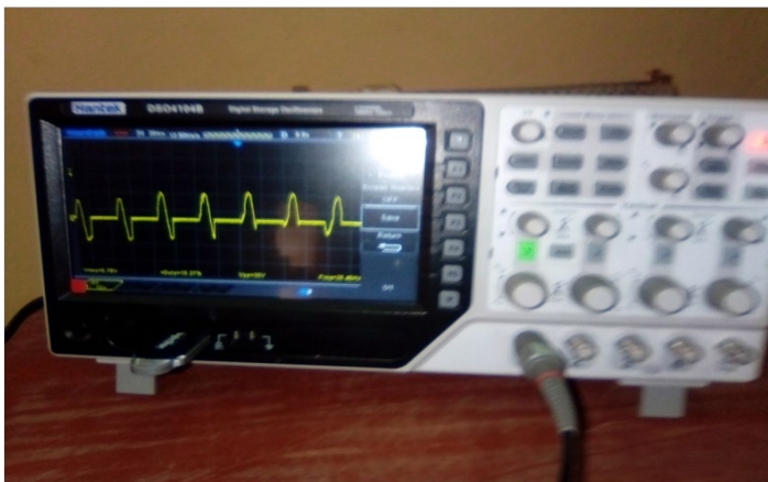
Figure 11. Oscilloscope display of inductance voltage wave form across 2/2 DSRM stator coil
