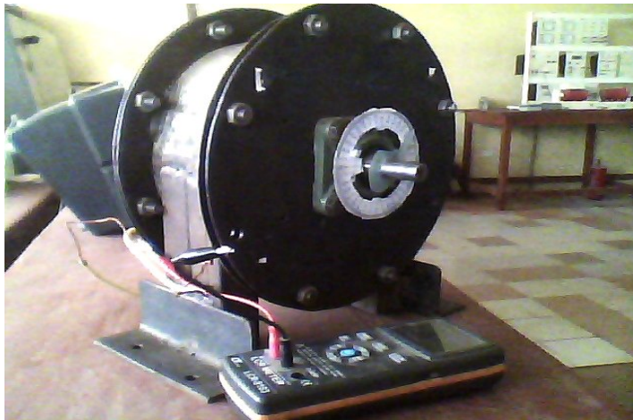
Figure 8. Experimental set up for inductance measurement using LCR meter
