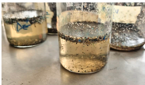
Fig. 2. Microplastics floating in beaker during extraction process.
