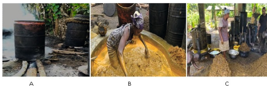
Fig. 4 Images showing traditional palm oil processing in Nigeria. A Boiling of oil palm fruit in a large drum until softened; B Manual extraction of oil from the softened fruit and separation of sludge; C use of local machines to separate oil from sludge
