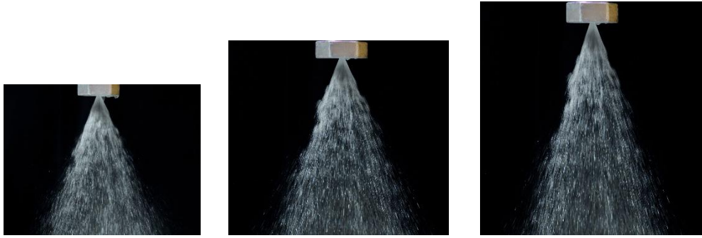
Figure 2: Spraying pattern of the nozzle at different heights
