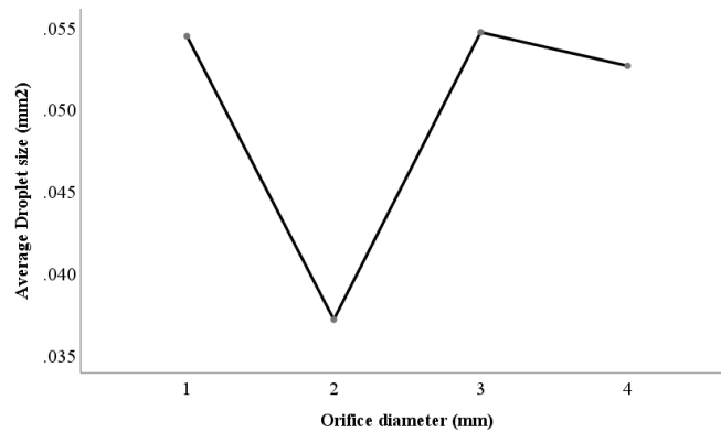
Figure 3: Effect of orifice diameter on average droplet size
