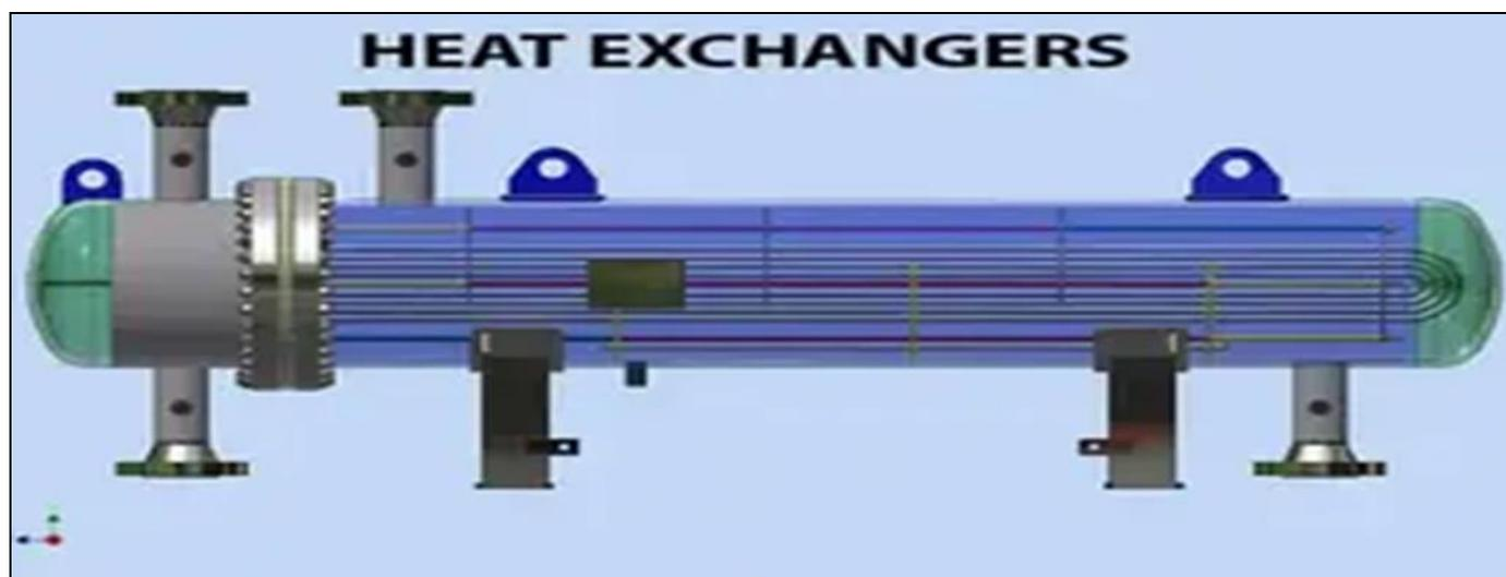
Fig 1 Shell and Tube Heat Exchanger [31]
