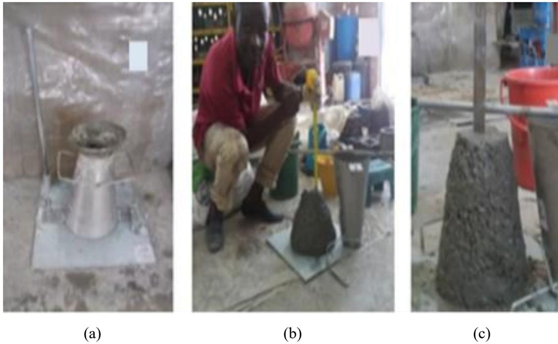
**Figure 1:** An Operational Procedure for Slump Test: (a) Abram's Slump Apparatus, (b and c) Measurement of Slump
