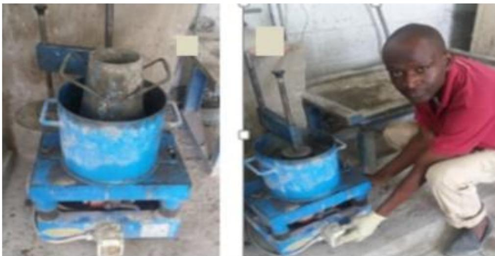
(a) Set up for Vebe test
