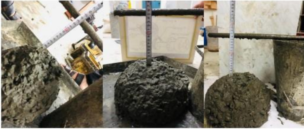
Plate 1: Slump test in progress
