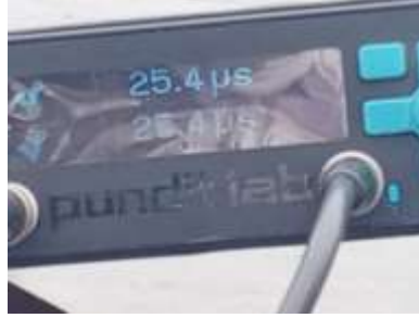
(b) Calibration of US meter
