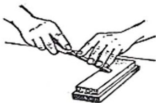
Fig. 8.7: Rubbing outside bevel on oil stone
