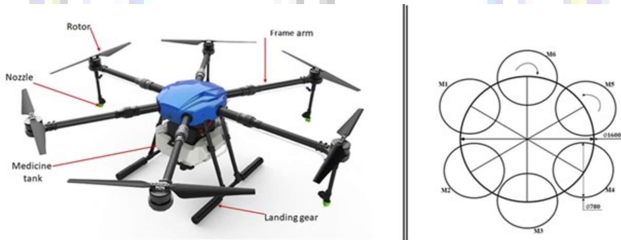
Figure 1: The Oryctes 16L drone, its propeller layout and sizing
