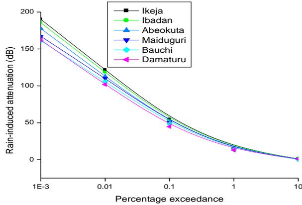
Figure 12: Rain-induced attenuation at 40 GHz uplink, vertical polarisation
