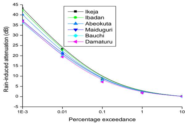
Figure 10: Rain-induced attenuation at 14 GHz uplink, vertical polarisation
