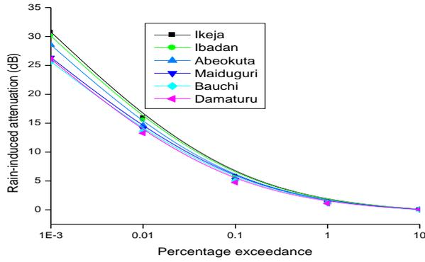
Figure 1: Rain-induced attenuation at 11 GHz downlink, horizontal polarisation
