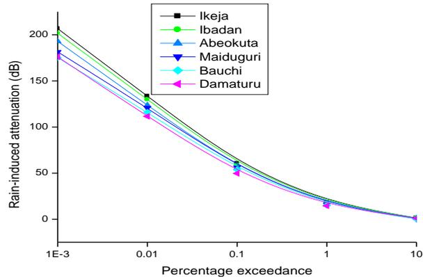
Figure 4: Rain-induced attenuation at 40 GHz uplink, horizontal polarisation
