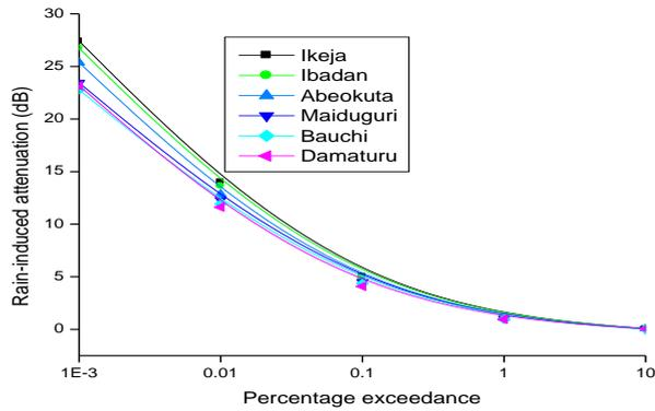
Figure 9: Rain-induced attenuation at 11 GHz downlink, vertical polarisation
