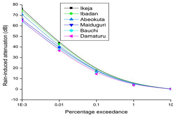
Figure 11: Rain-induced attenuation at 20 GHz downlink, vertical polarisation
