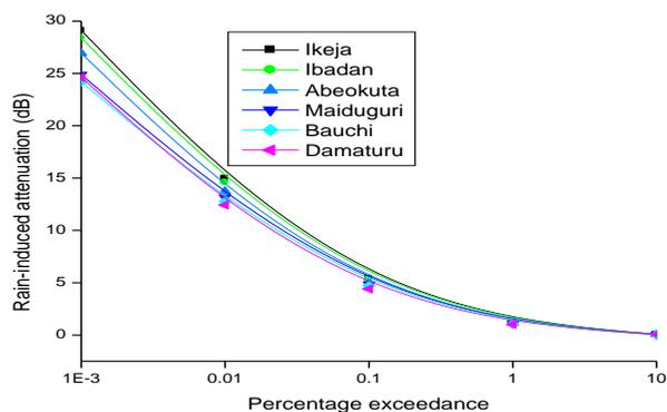
Figure 5: Rain-induced attenuation at 11 GHz downlink, circular polarisation
