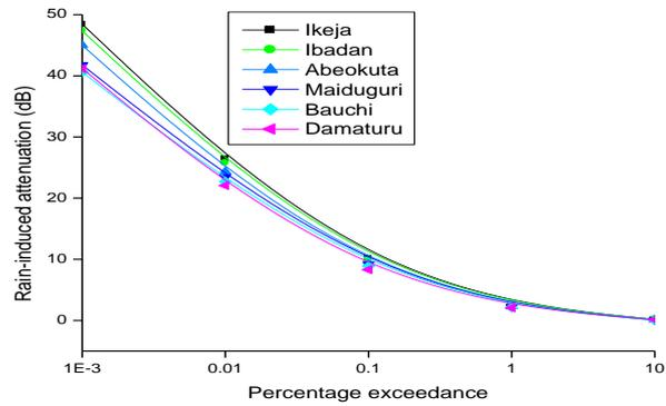
Figure 2: Rain-induced attenuation at 14 GHz uplink, horizontal polarisation
