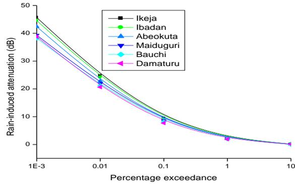
Figure 6: Rain-induced attenuation at 14 GHz uplink, circular polarisation
