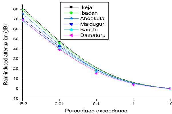
Figure 7: Rain-induced attenuation at 20 GHz downlink, circular polarisation
