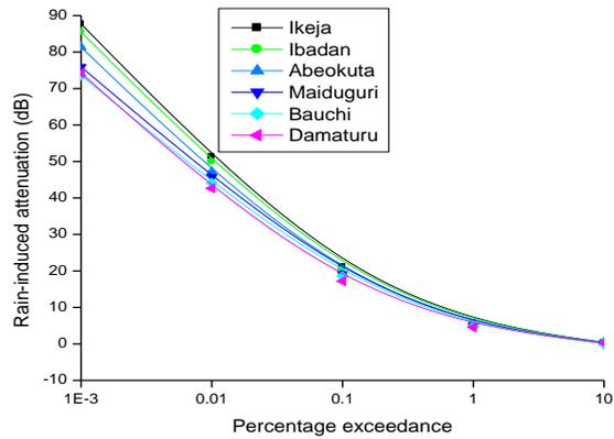
Figure 3: Rain-induced attenuation at 20 GHz downlink, horizontal polarisation
