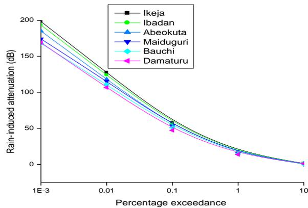
Figure 8: Rain-induced attenuation at 40 GHz uplink, circular polarisation
