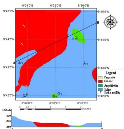
**Figure 9:** A geological map and cross section map (profile A-B) of the Saigbe area
