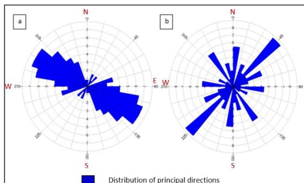
**Figure 7:** Principal joint directions in granite outcrops (a) and schist outcrops (b) from Saigbe area.
