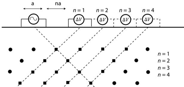
Figure 3. Illustration of dipole-dipole array pseudo-section when putting the measured values (Wahyu, 2016)
