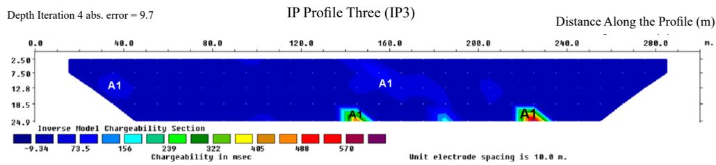
Figure 11. Inverse model chargeability section for profile three (IP3)
