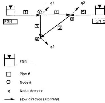
Figure 2. Typical Setup of Water Distribution Network
