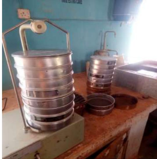
**Plate I Sieves used for the experiment**
