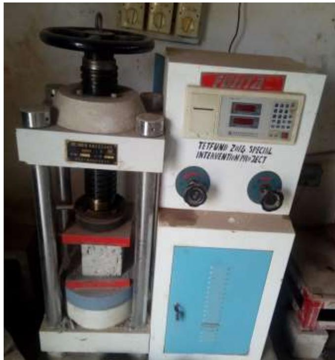
**Plate II Compressive strength test machine.**
