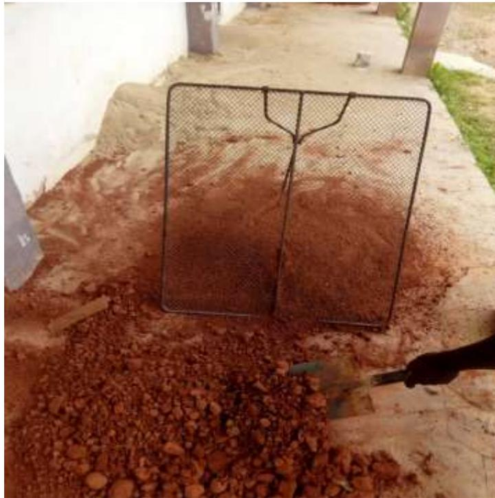
**Plate V: Sieve laterite using 5mm net**
