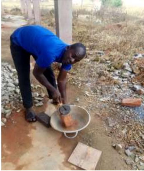
**XI Abrasion test of the brick**
