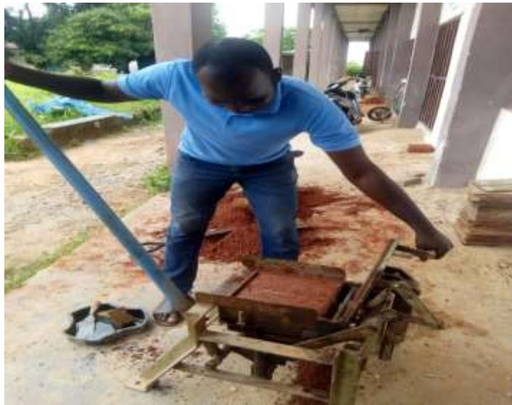
**Plate VII Moulding of brick with compressed manual machine**
