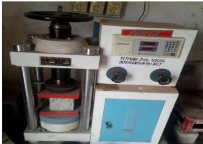
**Plate II: Compressive Strength Test Machine**
