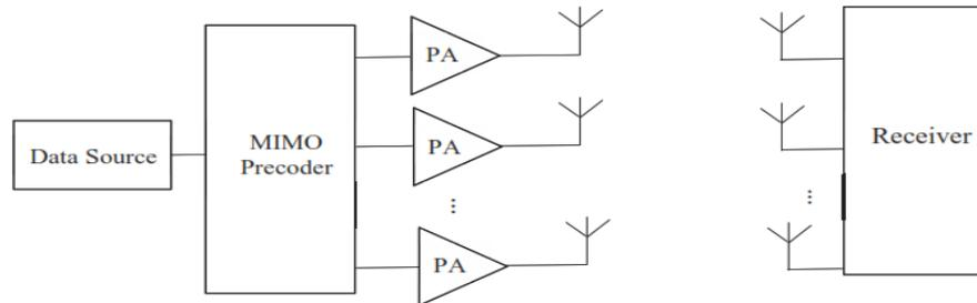
Figure 1. Multiple Input Multiple Output (MIMO) Structure
