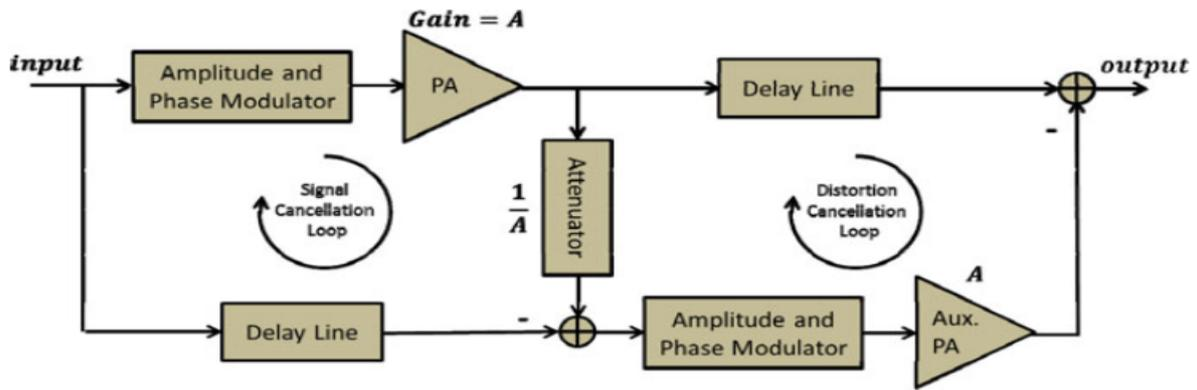
Figure 7. Block Diagram of Feedforward Linearization Technique (Cheaito, 2017).
