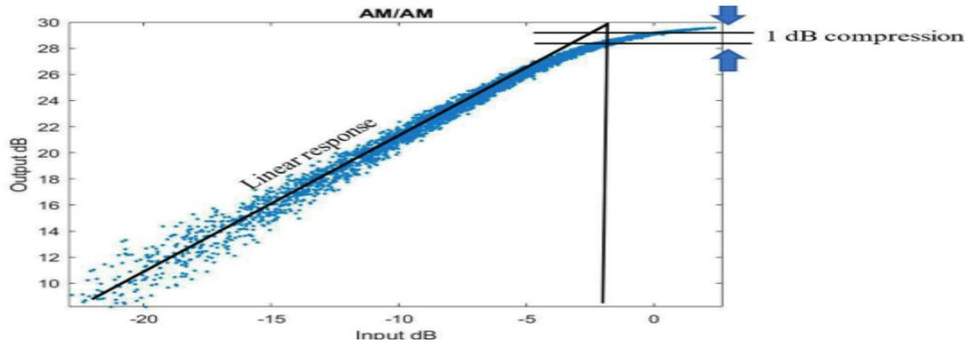
**Figure 4.** Power Amplifier Output Response.
