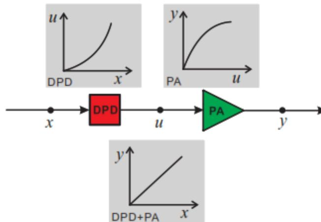
Figure 9. Principles of Pre-distortion Method (Guan & Zhu, 2017).
