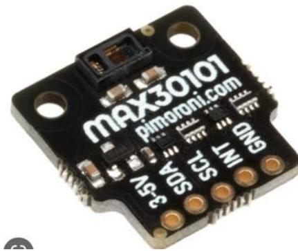
Figure 5: MAX30101 HR and BP sensor
