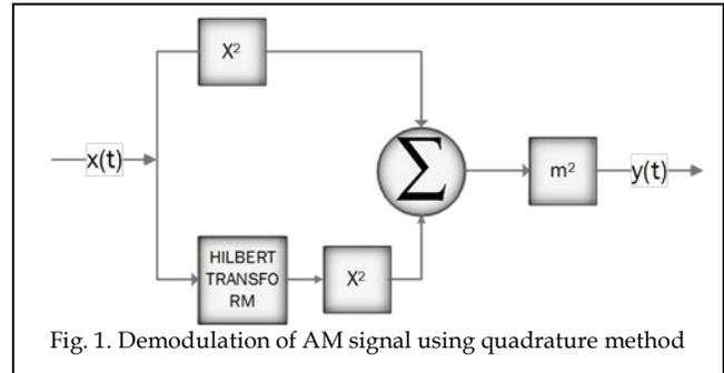
Fig. 1. Demodulation of AM signal using quadrature method
