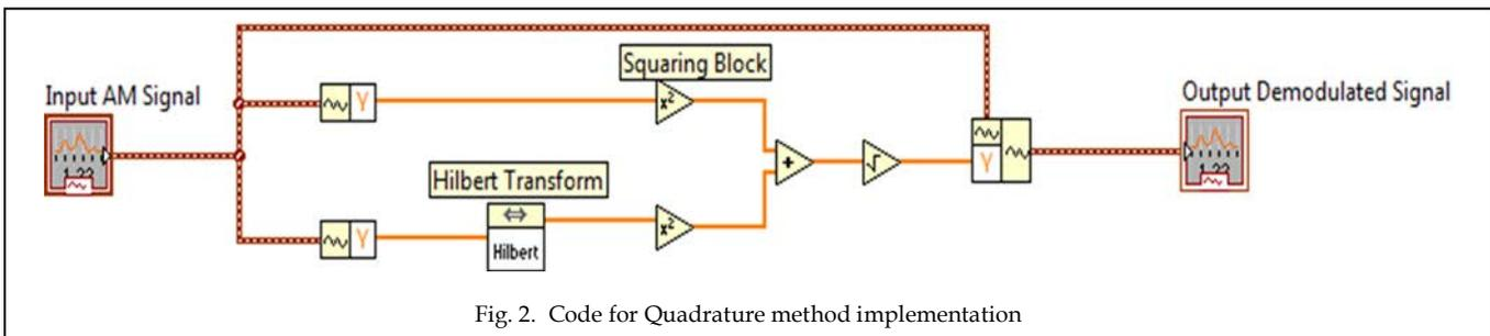
Fig. 2. Code for Quadrature method implementation
