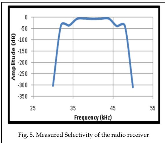
Fig. 5. Measured Selectivity of the radio receiver
