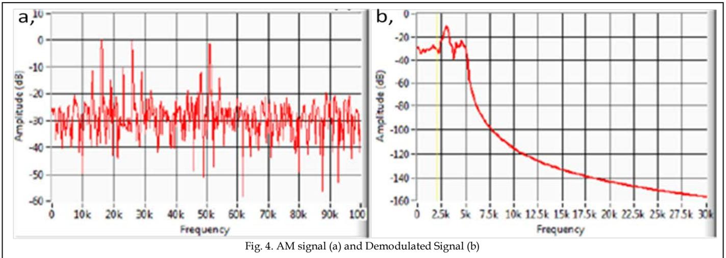
Fig. 4. AM signal (a) and Demodulated Signal (b)
