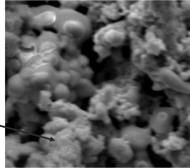
Pelleting and sintering at 1100 °C enabled trace phases like SrMoO and FeNiO to diffuse into the desired perovskite crystal structure.
