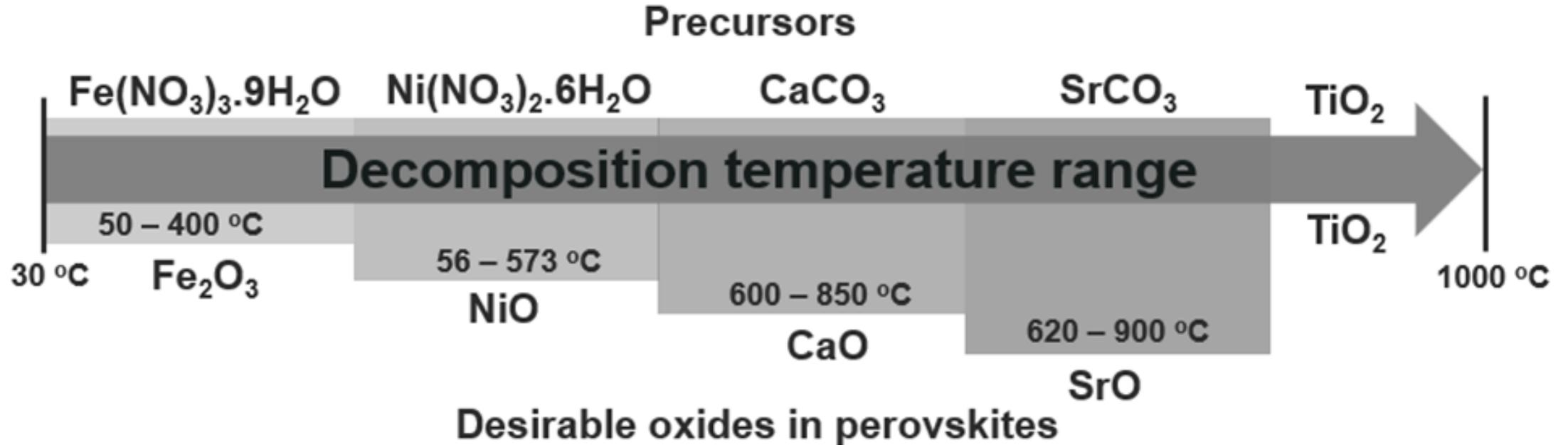
Key findings from TGA of the precursor materials, predicting 1000 °C as the calcination temperature for the novel perovskite
