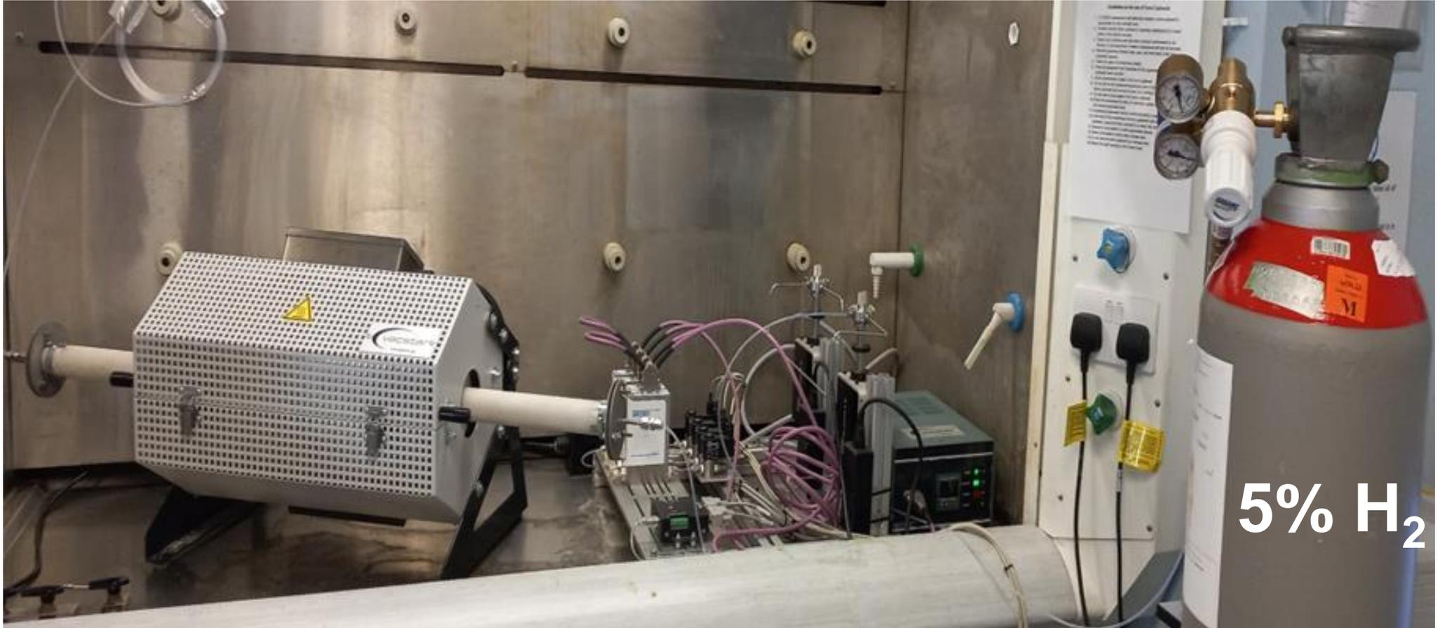
A reduction furnace set up for exsolution analysis, recently setup by our research group
