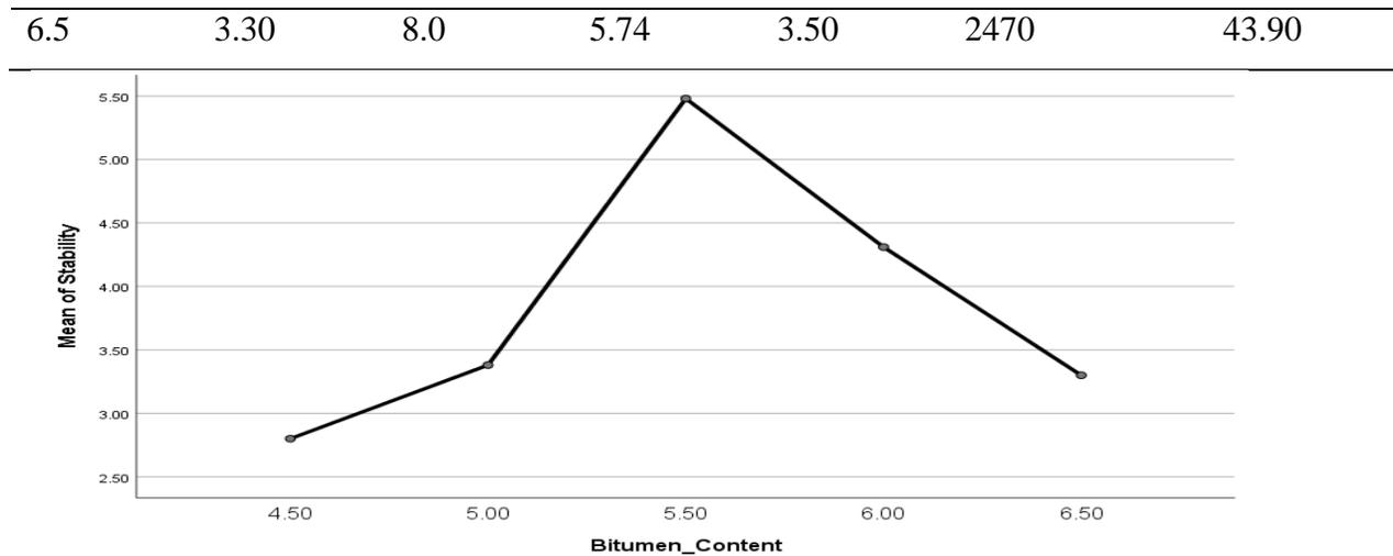
**Figure 2: Stability Versus Bitumen content**
