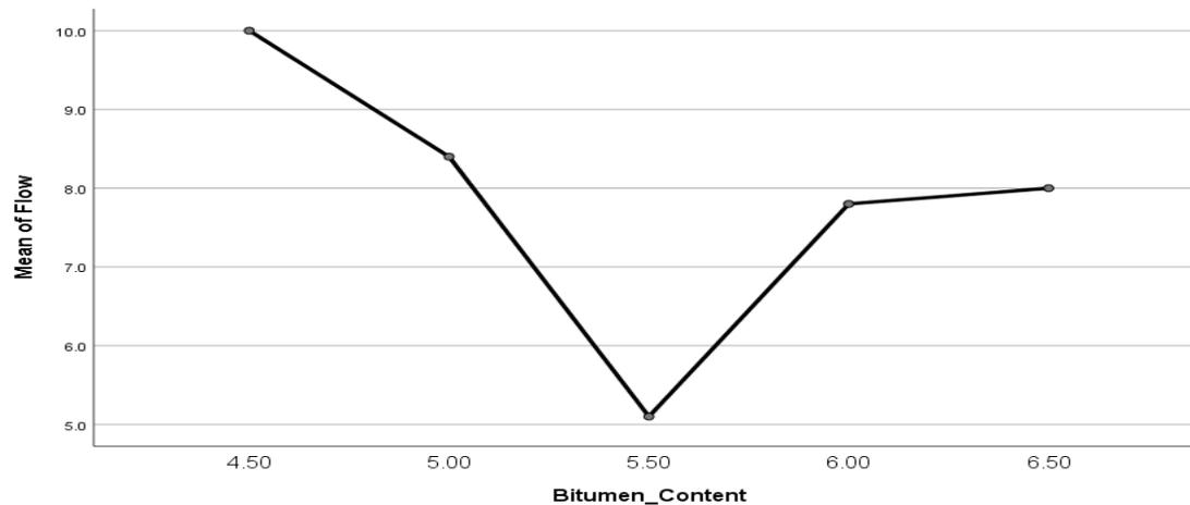
**Figure 3: Flow versus Bitumen content**
