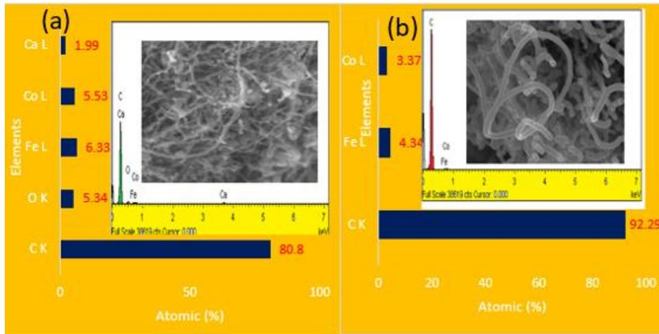
**Figure 6:** SEM/EDS of (a) as-produced and (b) purified MWCNTs showing the atomic % composition of each element in the samples
