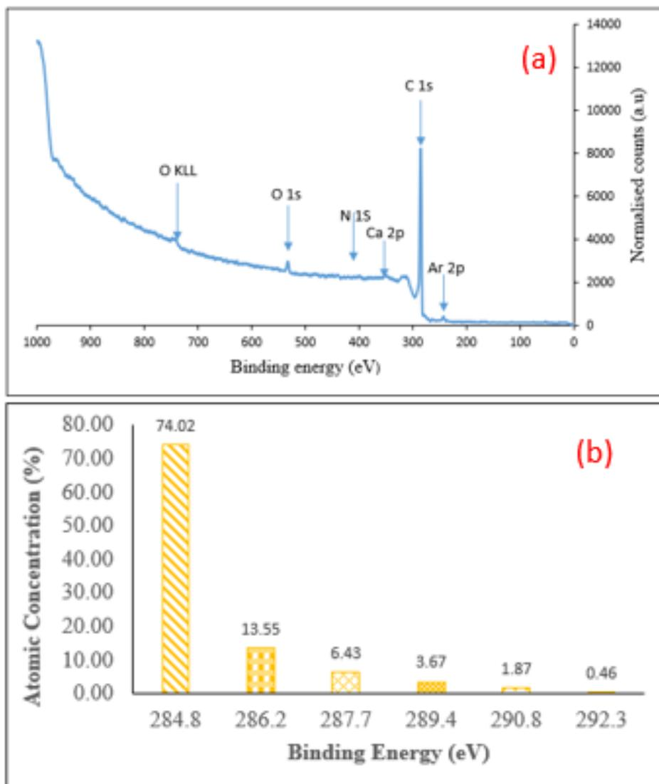
**Figure 9:** (a) XPS Scan of purified MWCNTs (b) Atomic % concentration of C 1s region for purified MWCNTs
