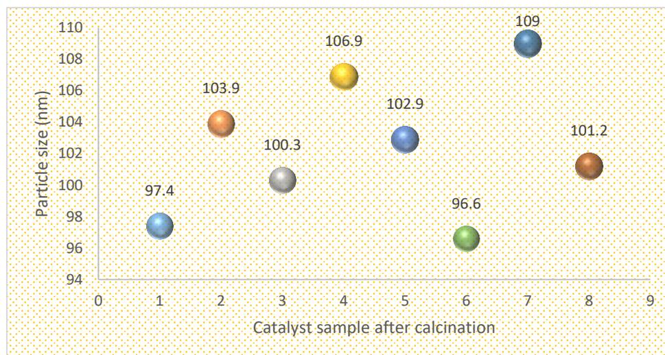
**Figure 3:** Catalyst particle sizes after calcination at 400 °C and grinding
