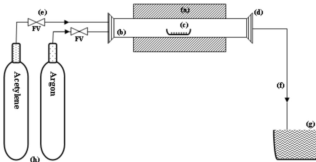
**Figure 1:** Scheme of set-up for CNT synthesis in CVD, (a) Furnace, (b) Quartz tube, (c) Ceramic boat with catalyst, (d) Cork, (e) Flow controller, (f) Gas outlet, (g) Gas collector with water, (h) Acetylene and Argon gas cylinders.
