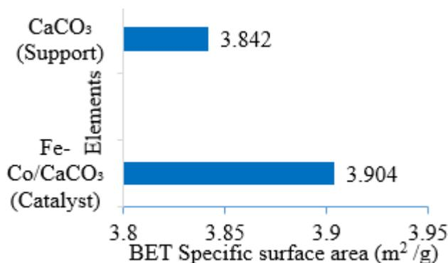
**Figure 2.** Surface area of CaCO<sub>3</sub> and Fe-Co/CaCO<sub>3</sub> catalyst
