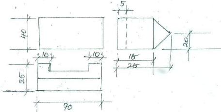
Q.3 )a Draw the block in Isometric projection and its views in first angle
