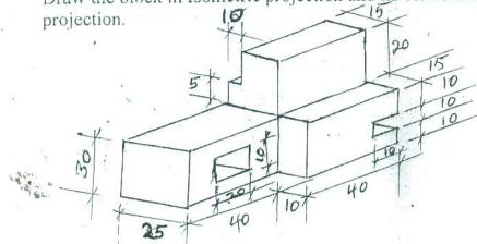
Q. 4(a) Construct the block given and its elevations in third angle projection. Use scale: 2:1.
