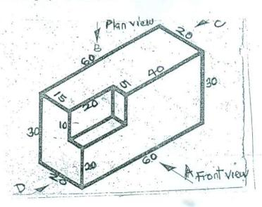
With the aid of the object above, produce the first and third angle projection of the block. (20 marks)
