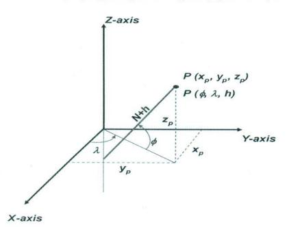
(ii). Given the geodetic coordinate of P as  $\phi = 10^{\circ}$  30' 30'',  $\lambda = 06^{\circ}$  15' 25'' and h = 239.630m on Clarke 1880 ellipsoid with parameters a = 6378249.145m and 1/f = 293.465. Determine the cartesian coordinate of  $P(X_p, Y_p, Z_p)$ . Hint:  $N = \frac{a}{(1-e^2\sin^2\varphi)^{\frac{1}{2}}}$ ,  $e^2 = \frac{a^2-b^2}{a^2}$  (10 marks)
