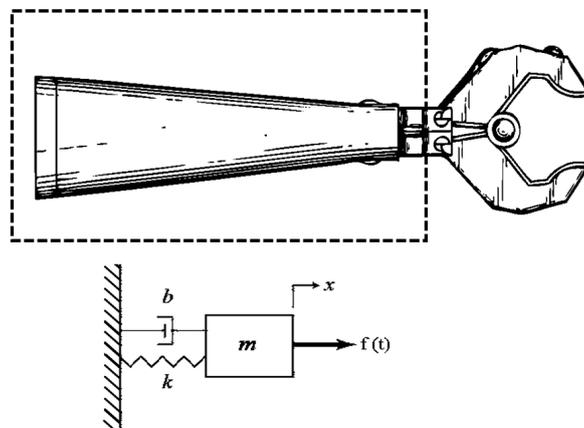
Figure Q1: 1 DOF Robot Arm
