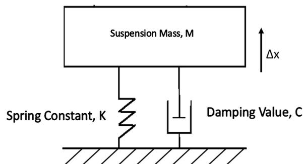
Figure 1: Suspension Model
