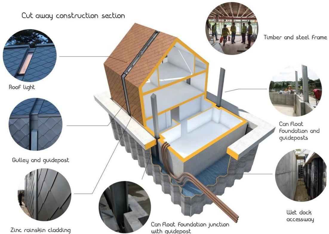
Figure 2.1: Showing Cut out section of The Thames Amphibious House
