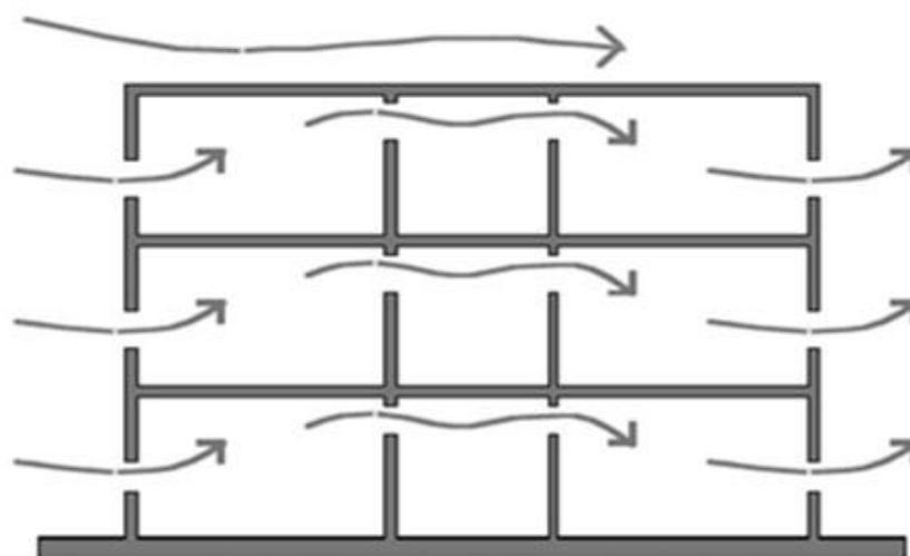
Figure 2.2. The line diagram of wind driven cross-ventilation
