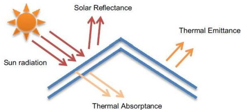
Figure 2.11. Showing Cool roof mechanism
