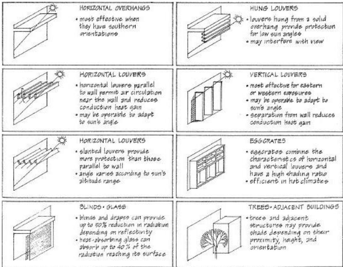
Figure 2.6. The various forms of shading devices
