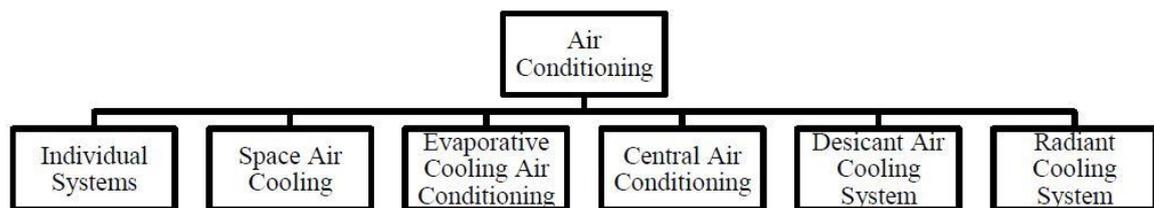
Figure 2.5. Categorization of air-conditioning systems
