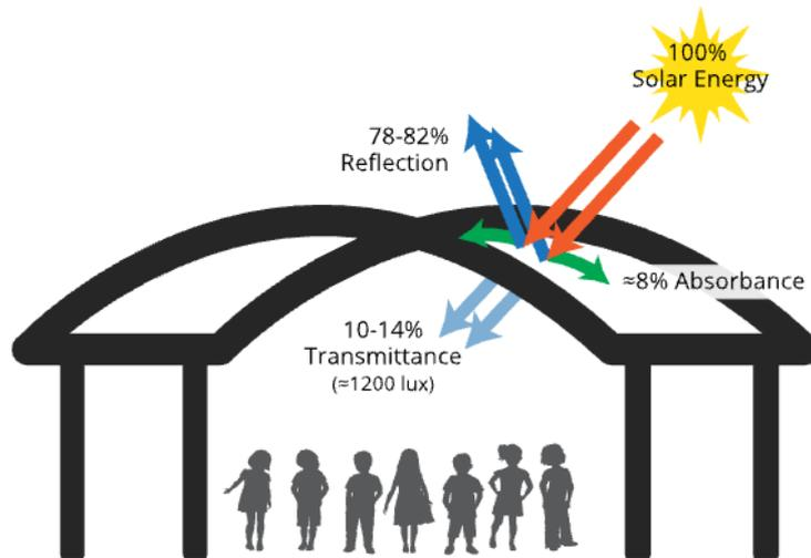
Figure 4.18: An illustration of how PTFE works.
