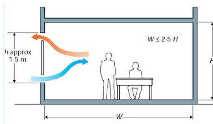
Figure 2.3: Inflow of fresh cool air and outflow of polluted air on a single-sided space.
