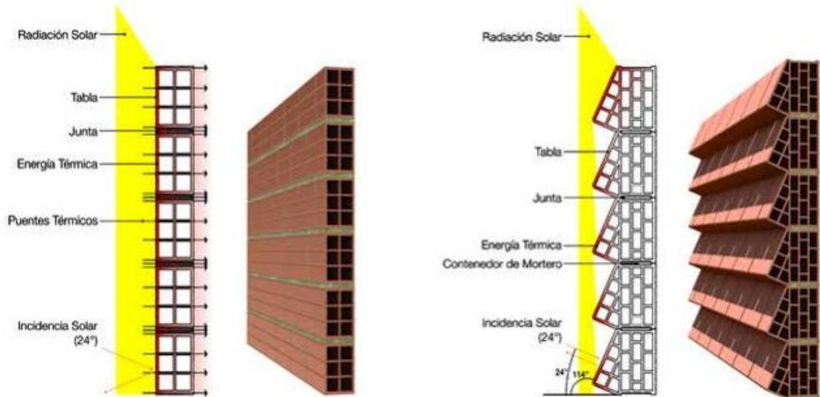
Figure 2.9. Bricks at an angle reducing the area exposed to solar radiation
