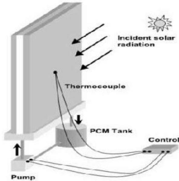
Figure 2.8. Experimental test rig of Phase Change Material filled wall board
