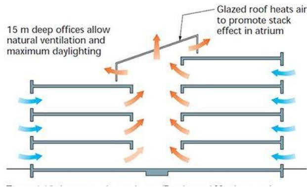
Figure 2.4: Inflow of fresh cool air and outflow of polluted air through a stack ventilation process.
