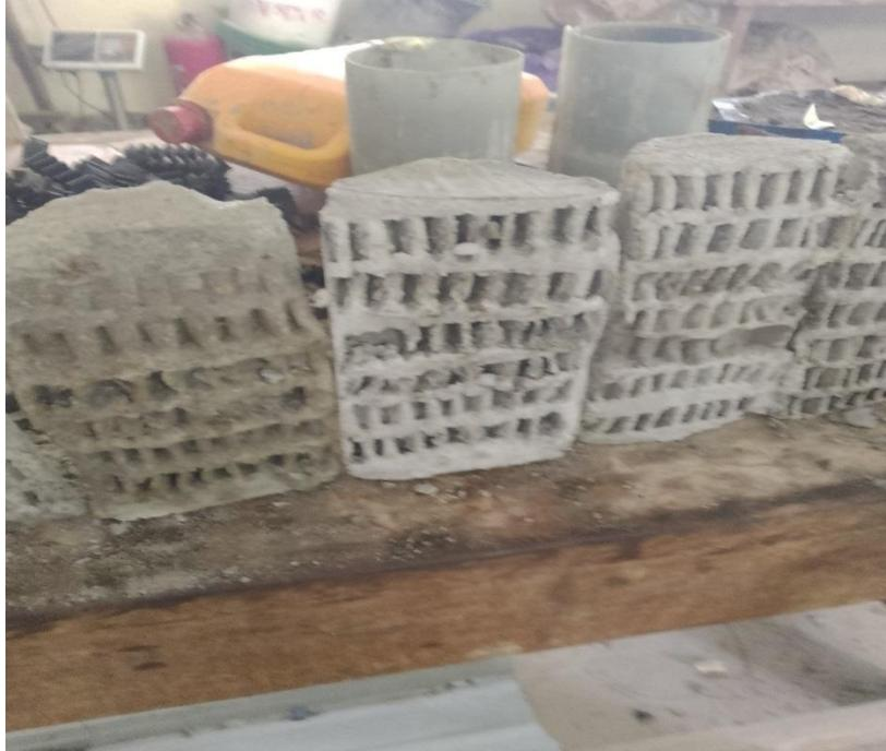
**Plate 3.3: Cast Interlock bond Specimens**
