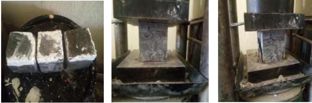
**Plate VII: compressive strength test setup, withdrawal of samples from the curing tank (left), loaded sample (middle), and sample at failure state (right)**
