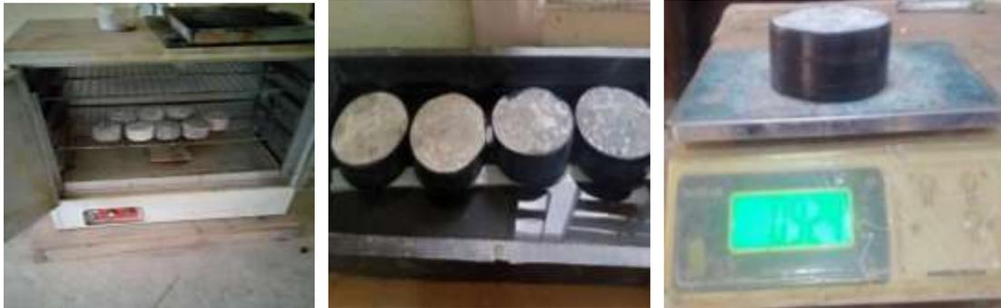
**Plate VIII: Sorptivity test setup, drying of samples (left), samples exposed to capillary action in the water (middle), and sample weighing (right)**
