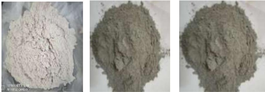
**Plate I: Silica fume (left), Millet husk ash (middle) and Portland cement ((Right)**
