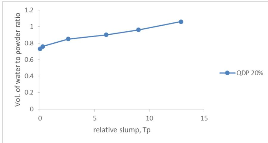
**Figure 4.6: Volume of water to powder ratio versus relative slump for 20 % QD mix**
