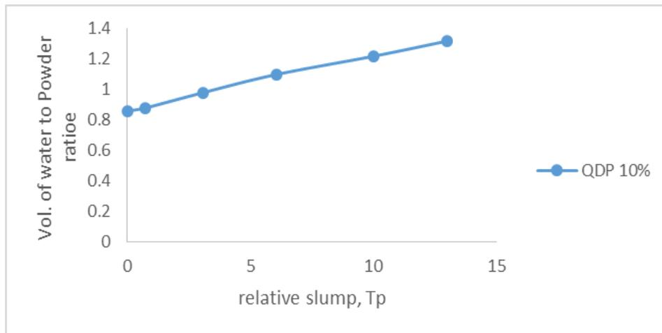
**Figure 4.5: Volume of water to powder ratio versus relative slump for 10 % QD mix**
