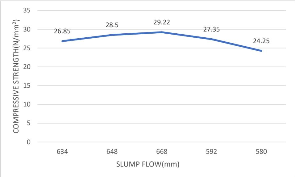
**Figure 4.8: Compressive strength at 28 days versus the slump flow**
