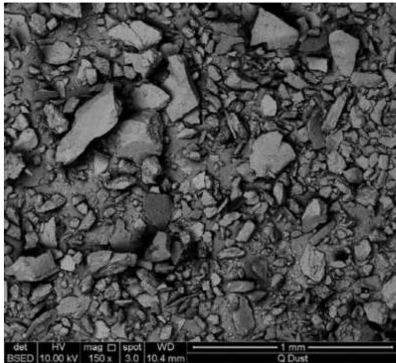
**Figure 4.2: Scanning electron microscopy (SEM) of QDP**
