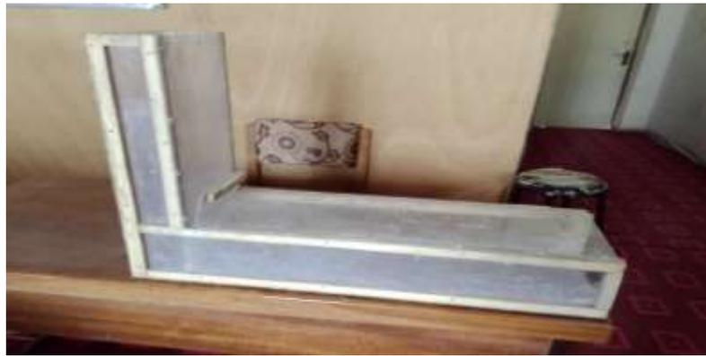
**Plate II: L – Box: used to measure passing Ability of the Mixes**
