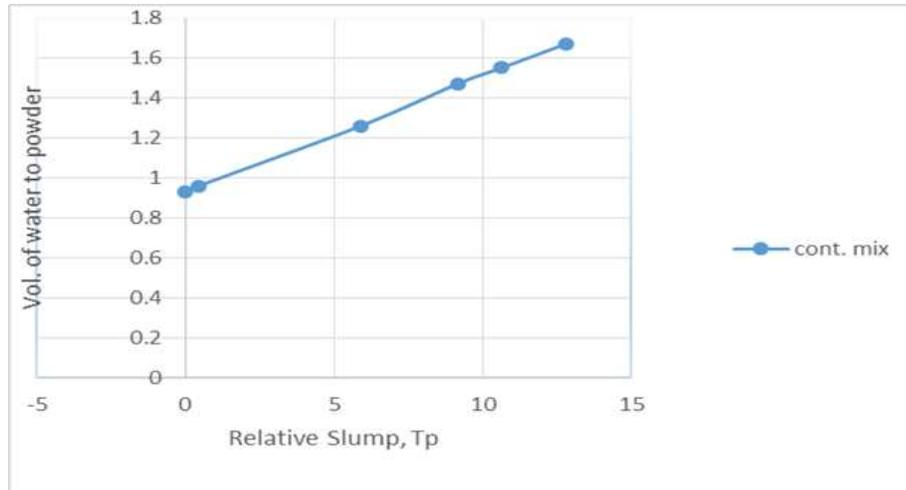
**Figure 4.4: Volume of water to powder ratio versus relative slump for PC mix**
