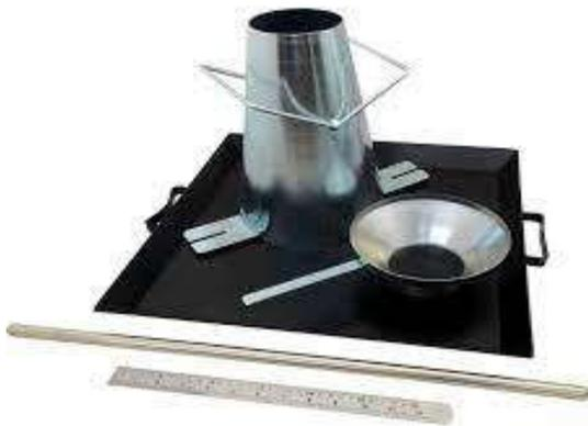
**Plate I: Slump cone: used to measure flowability of the Mixes**
