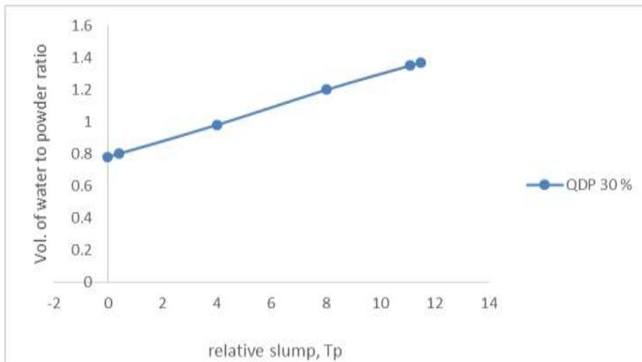
**Figure 4.7: Volume of water to powder ratio versus relative slump for 30 % QD mix**
