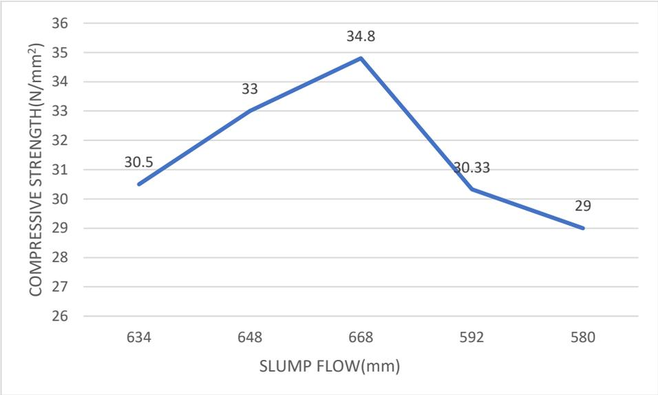
**Figure 4.9: Compressive strength at 56 days versus the slump flow**
