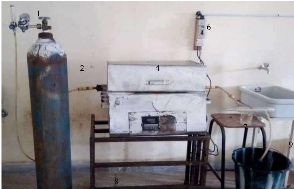
Plate V: Pyrolysis Experimental Set up
