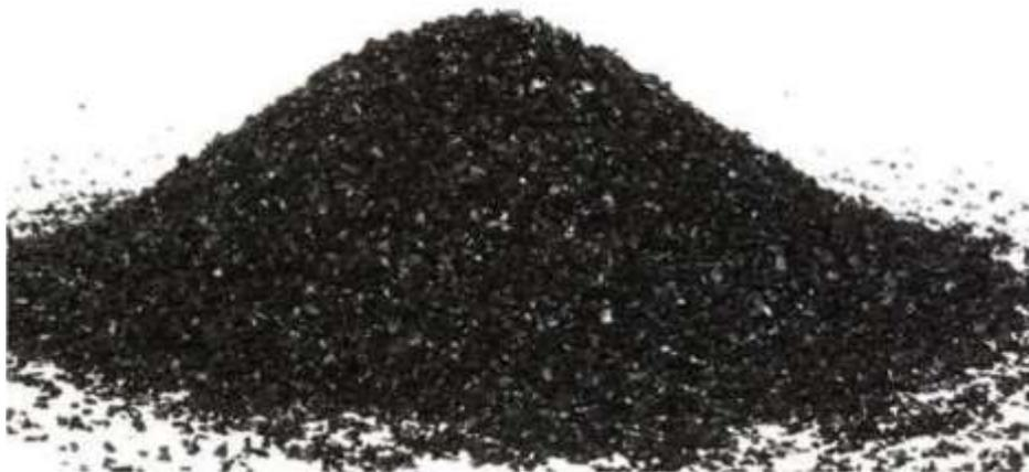
Plate III: Granular Activated Carbon (Foroutan et al., 2018)
