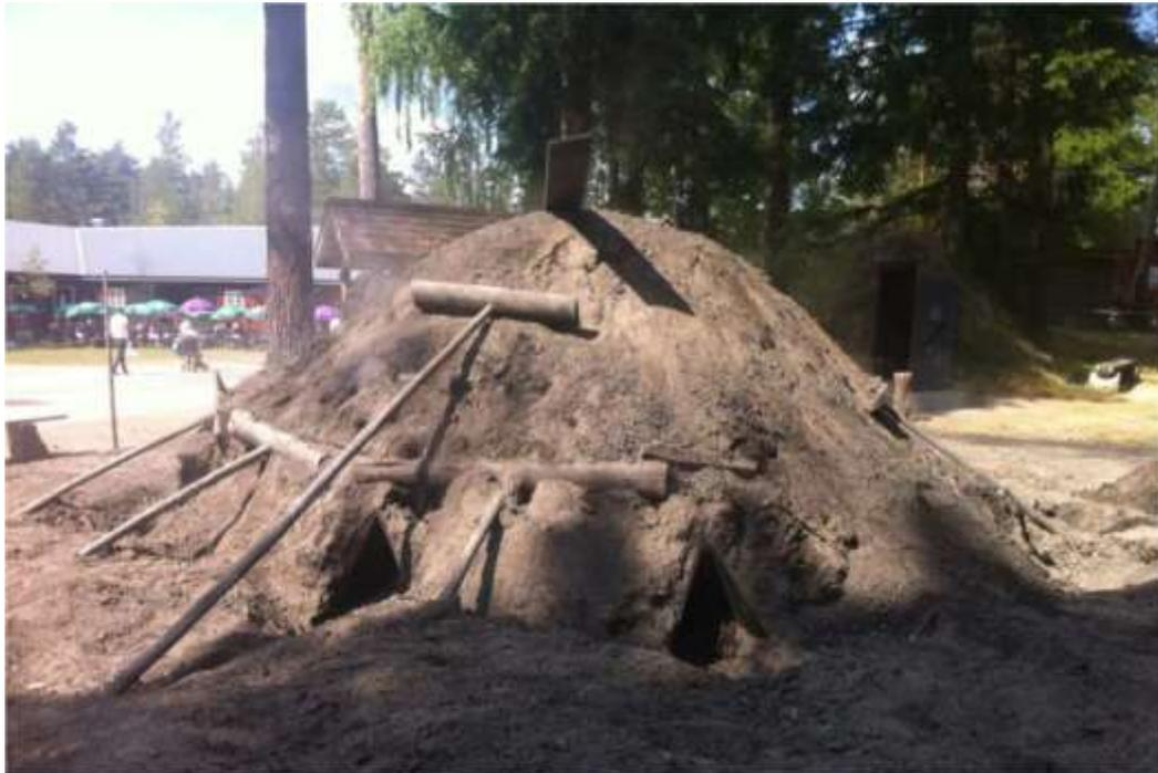
Plate I: Typical kiln Showing Production of Charcoal
