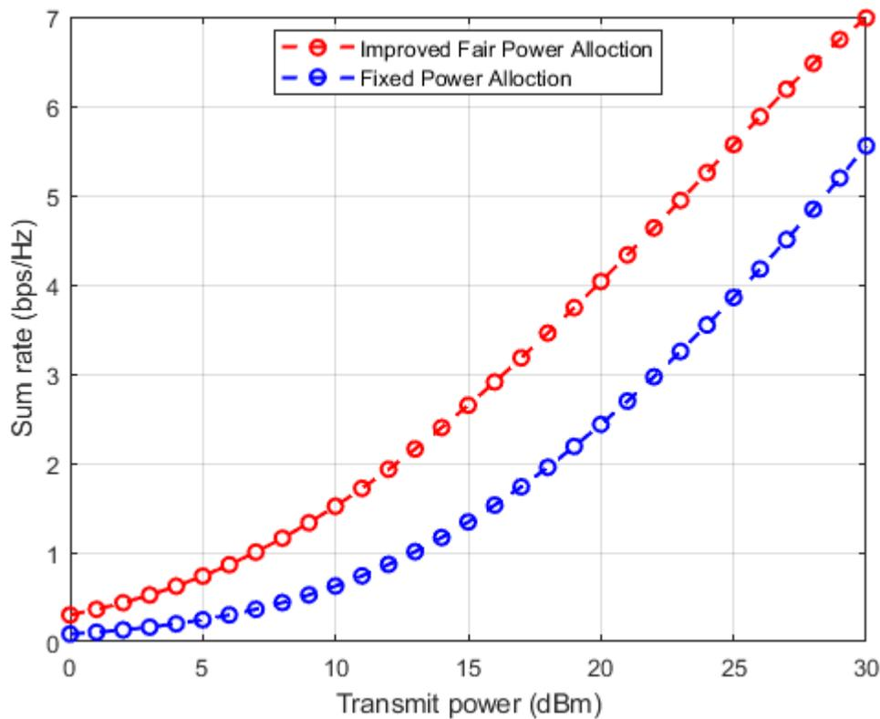
Figure 4. 6: Sum Rate vs. Transmit Power for the Improved Fair Power Allocation
