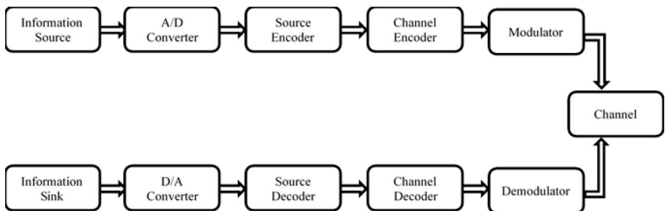
Figure 3. 3: A digital communication system's block diagram
