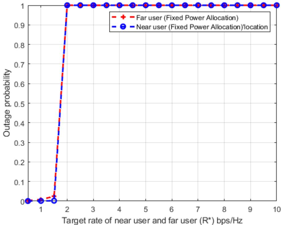
Figure 4. 1: Outage probability vs.  $R^*$  for Fixed Power Allocation
