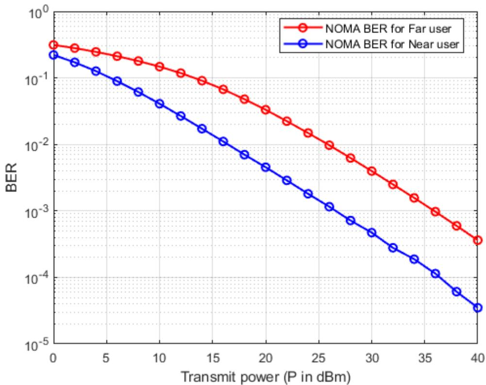
Figure 4. 5: BER Performance vs. Transmit Power (dBm)
