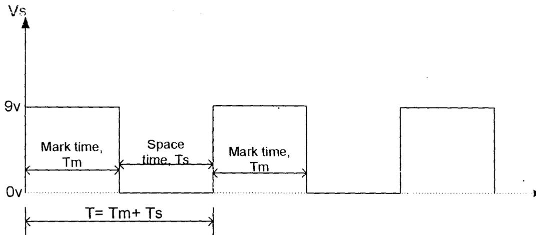
FIG 3.7 Square Waveform Output of a Warbling Siren
