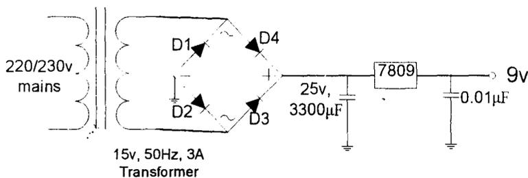
FIG 3.0 Power Rectification Process to 9v
