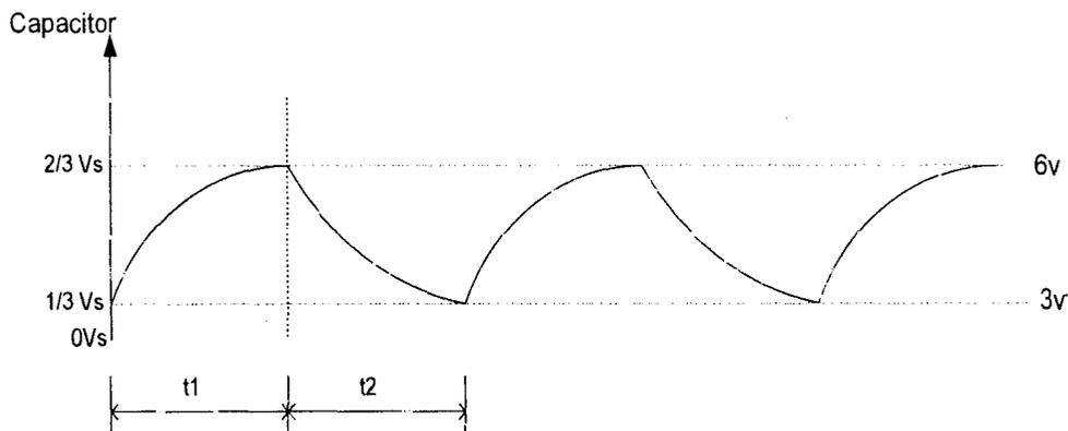
FIG 3.6 The Wailing Output Waveform of the Siren
