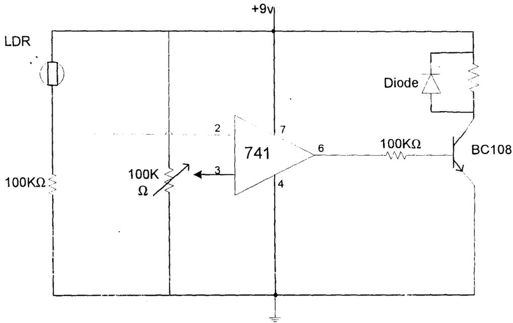
FIG 3.5 The LDR circuit diagram as used in this project.
