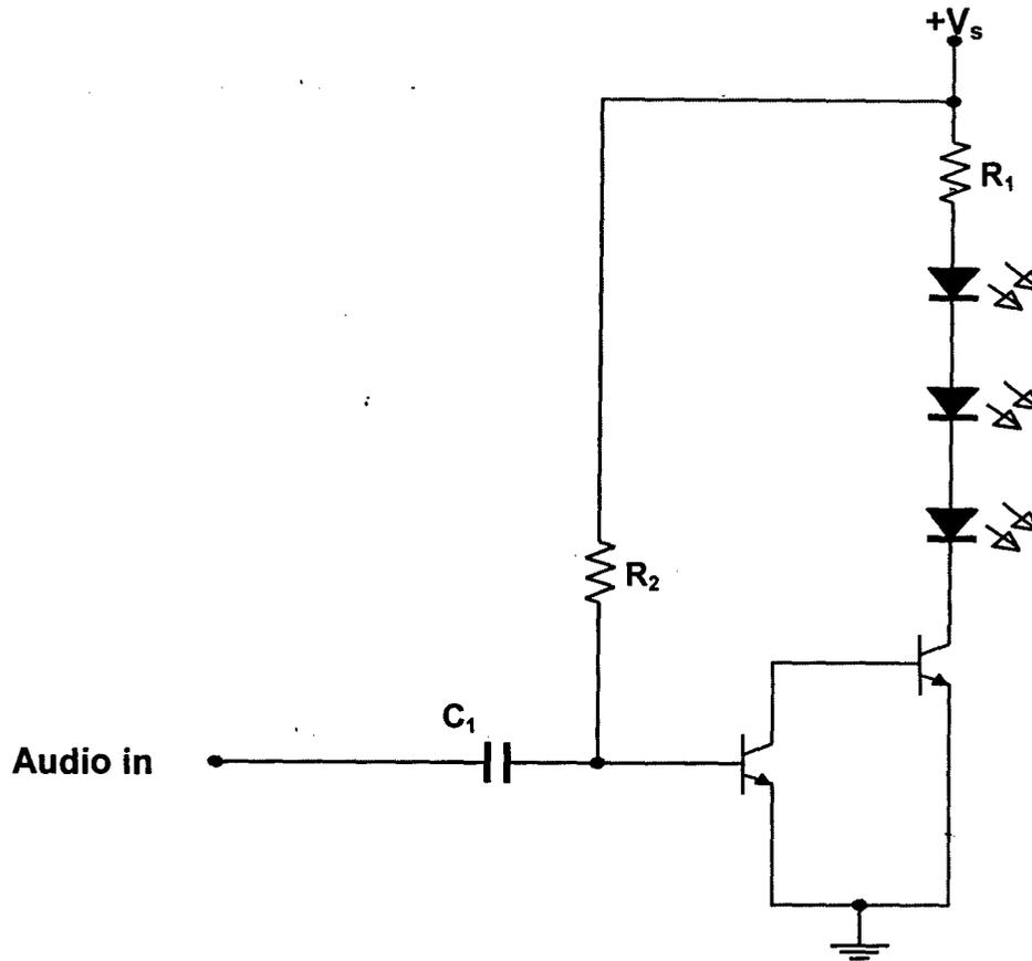
Fig 3.1 The transmitter stage
