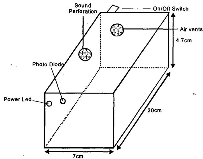
Fig. 4.3 Isometric view of receiver cased with dimensions
