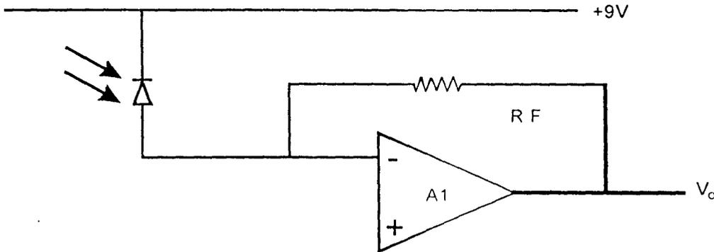
Fig. 3.3 (Photodiode and operational amplifier)
