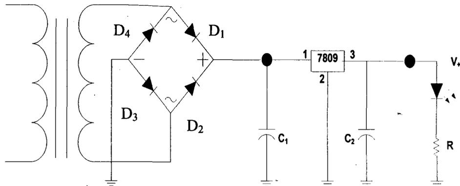
FIG. 3.5 Power supply circuit
