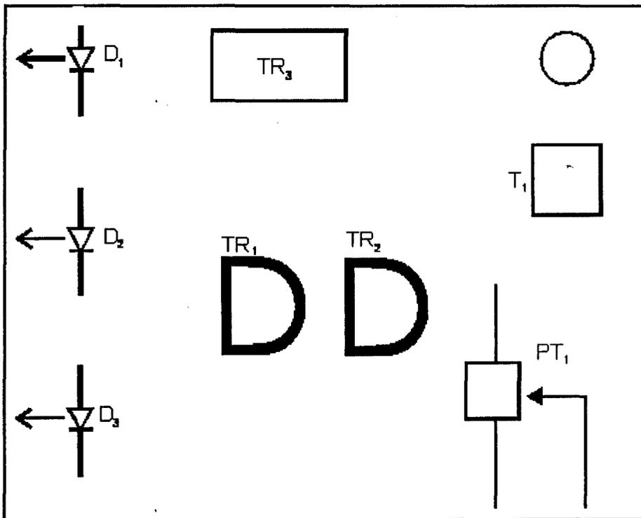
Fig. 4.0 Component layout of the transmitter on vero board
