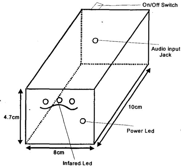
Fig. 4.2 Isometric view of transmitter cased with dimensions
