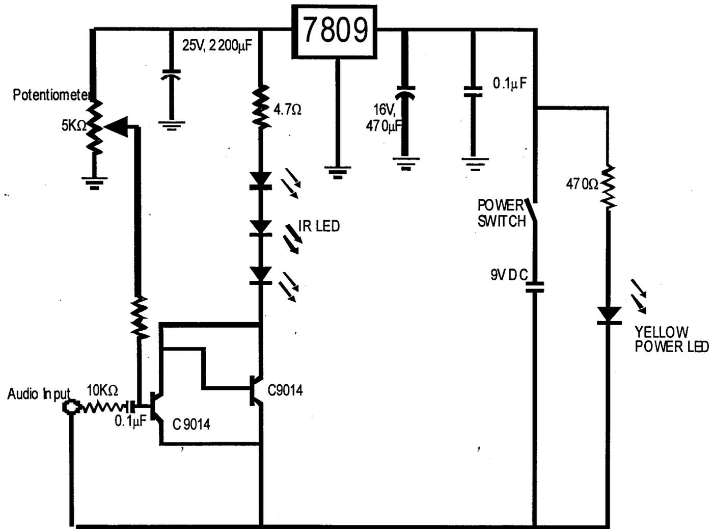
FIG. 3.7 CIRCUIT DIAGRAM OF TRANSMITTER
