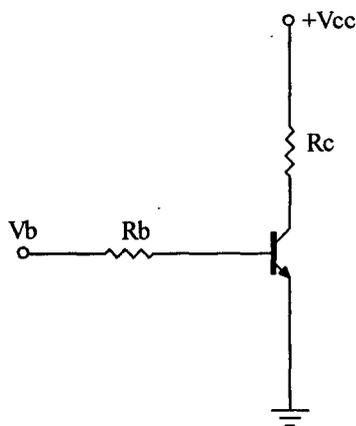
Fig 2.2 Transistor as a Switch
