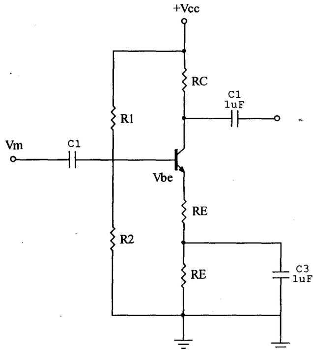
Fig 2.1 Transistor as an Amplifier
