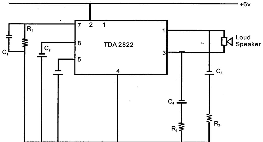
Fig. 3.4 Output stage circuit diagram
