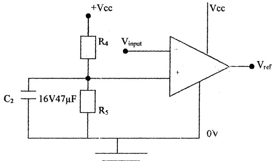
**FIG 3.3 SINGLE-SUPPLY BIASING OF AN OP-AMP**
