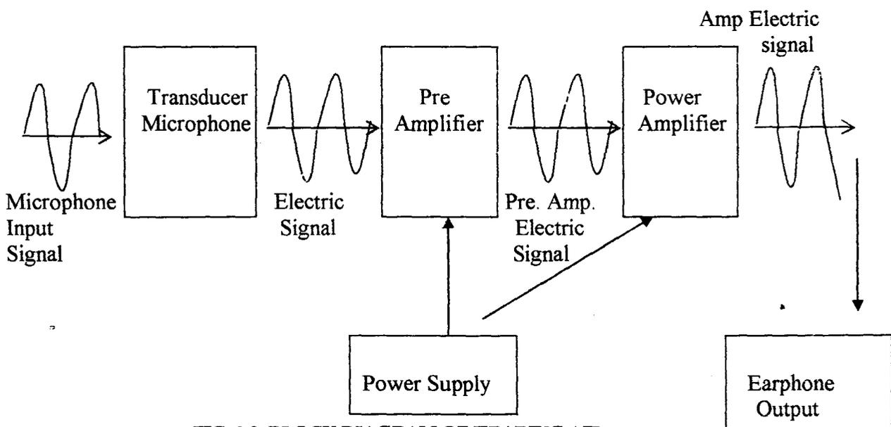
FIG. 2.2 BLOCK DIAGRAM OF HEARING AID
