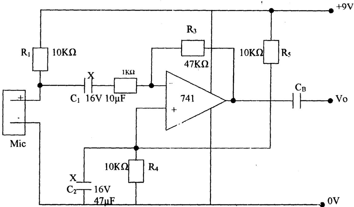
**Fig 3.1 Microphone Preamplifier**
