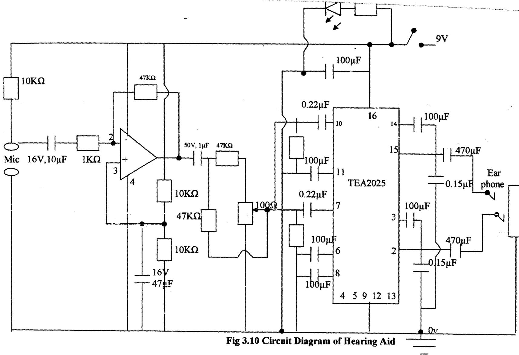
Fig 3.10 Circuit Diagram of Hearing Aid
