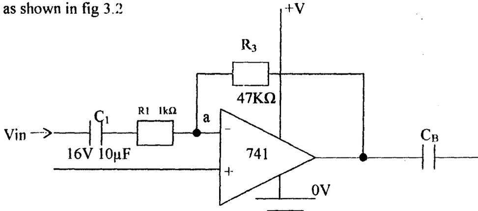
**Fig 3.2 741 inverting Op-Amp**
