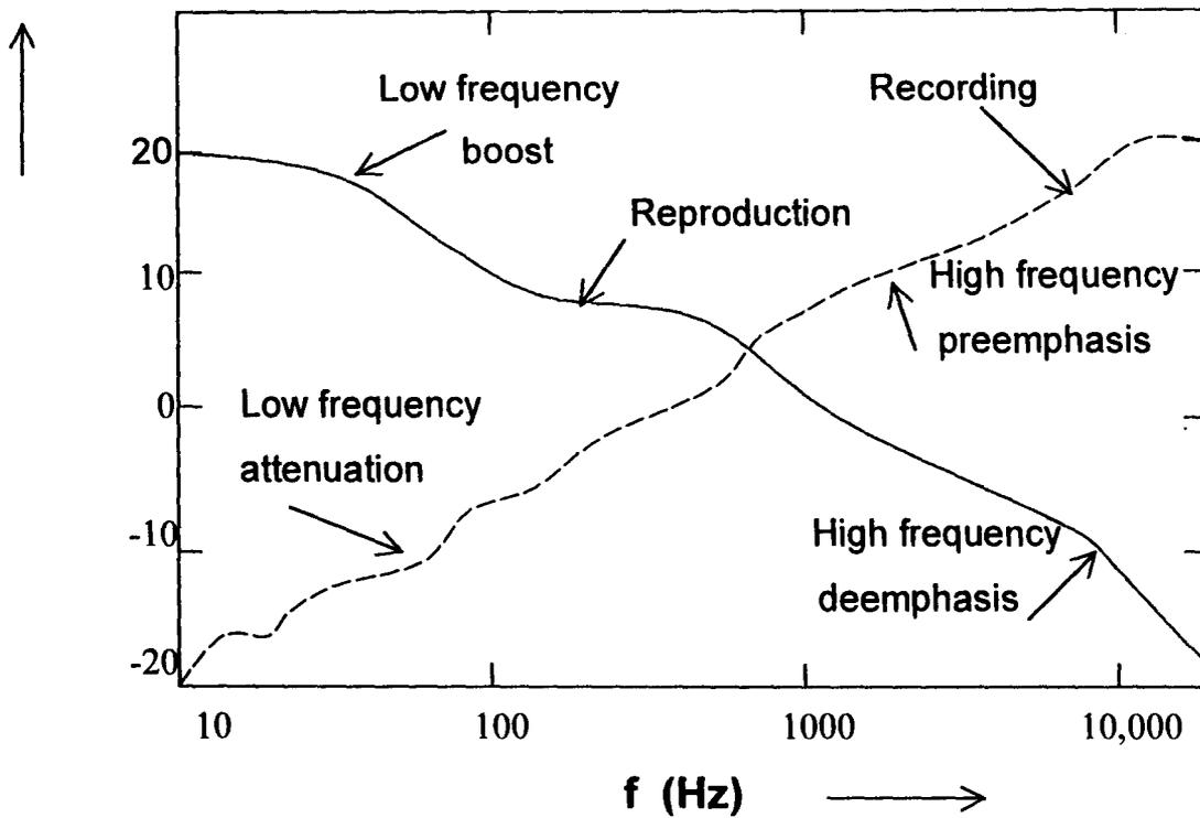
**Figure 1-3** Equalization curves for phonograph recording and playback
