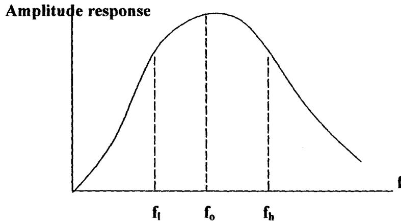
**Figure 2-2** The illustration of band-pass filter response.
