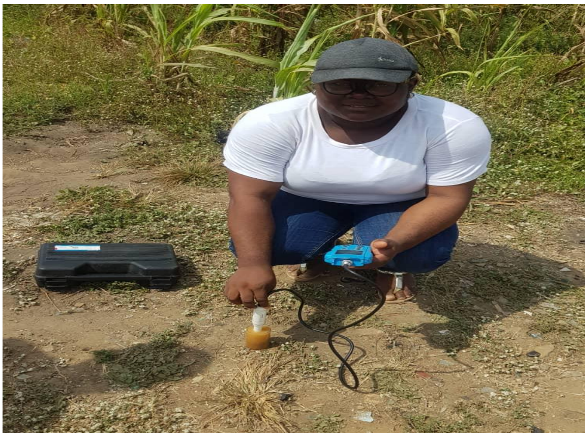
Plate IV: Insitu measurement of Physical Parameters using Multi-meter
