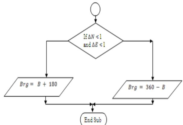
Figure 4: Chart Showing Subroutine for Bearing Reduction (Source: Authors' Research)
