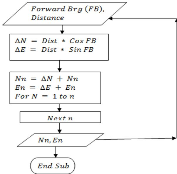
Figure 2: Chart Showing Subroutine for Forward Computation (Source: Authors' Research)
