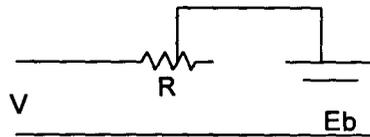
Figure 2: Constant voltage system
