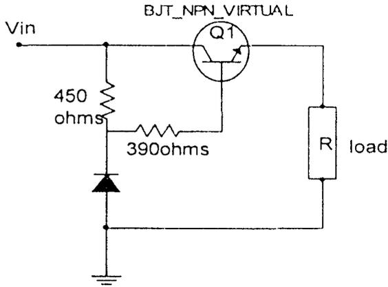
Figure 3.4: Series regulation circuit
