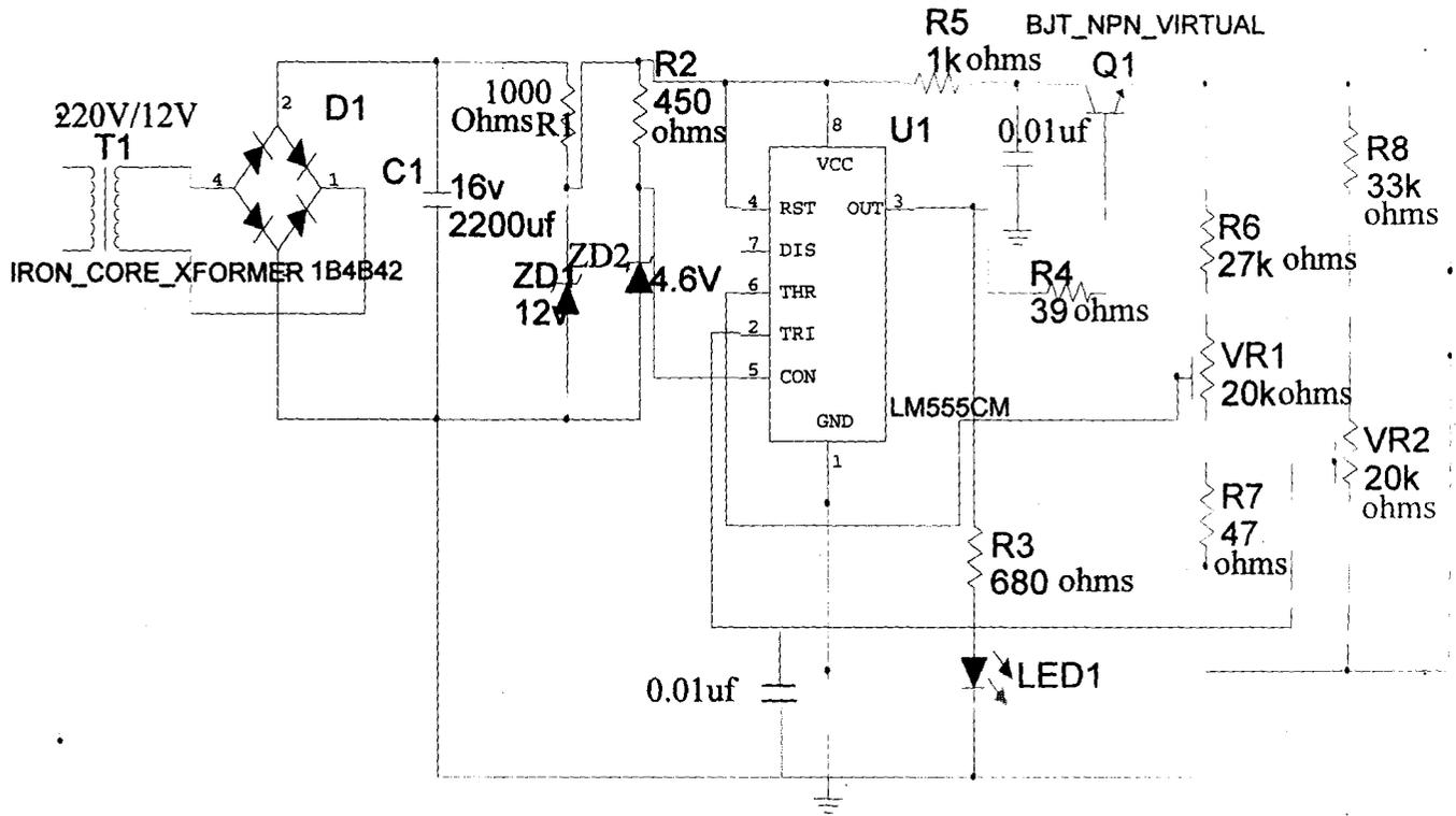
Fig. 3.9: Complete circuit diagram of a Nokia 1200 cell phone battery charger
