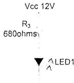
Figure 3.8: State of charge indicator
