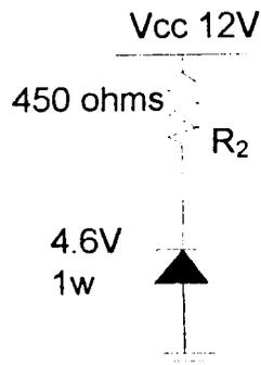
Figure 3.5: Diagram of a reference voltage
