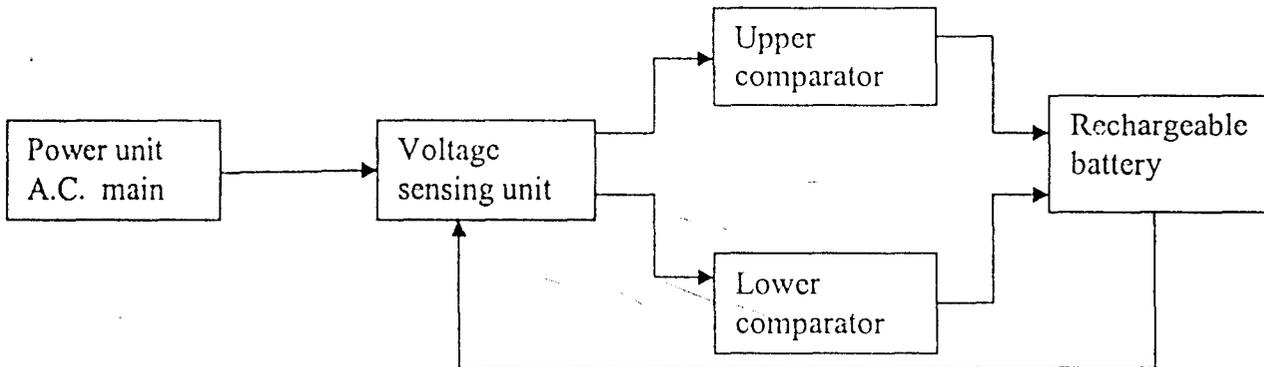
Figure 3.1: Block diagram of the circuit
