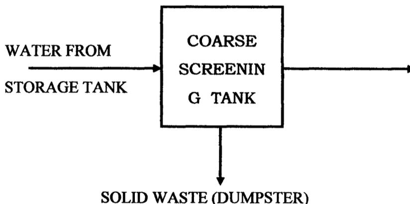
This is a primary process used to remove larger entrained objects ranging from 100 – 1000mm in size that are deposited in the waste water tank, such as rags, sticks,
