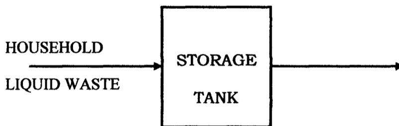
The raw water storage tank as shown above is a tank used to store waste water from different areas of the environment, such as household waste liquid from toilet, baths, showers, kitchens, sinks and so forth disposed off via sewers. The waste water is further transferred from the storage tank to the screening tank.
