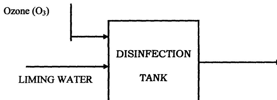
This is the last unit in the purification of domestic waste water treatment however, in this process ozonation takes place.
