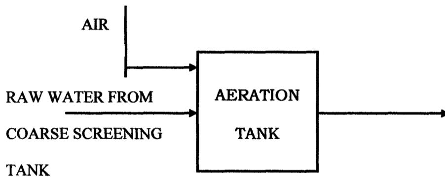
As it is applied to domestic waste water treatment, aeration can be defined as the process by which a gaseous phase usually air and water are brought into intimate contact with each other for the purpose of transferring volatile substances to or from the water. These volatiles substances include oxygen, carbohydrate, nitrogen, hydrogen sulphate, methane and various unidentified organic compounds responsible for taste and odour.
