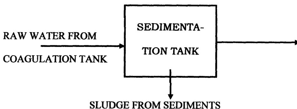
This process unit is used to reduce the amount of settleable solids by chemical treatment, such as the addition of coagulant to remove colour and turbidity, this unit is
