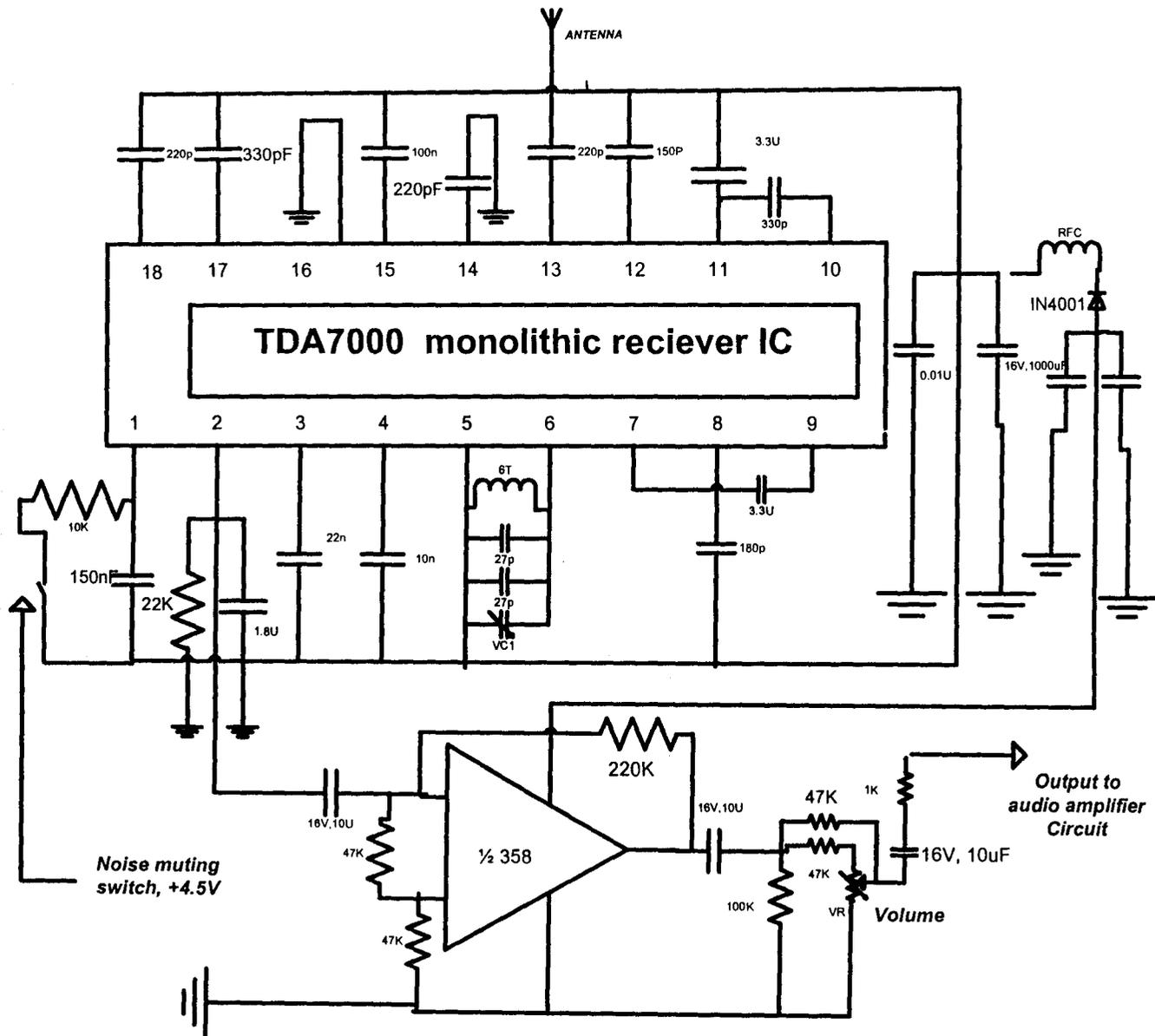
Fig.3.5 Circuit diagram of a TDA 7000 Frequency Modulation Receiver (all ground connection should terminate at pin 16)
