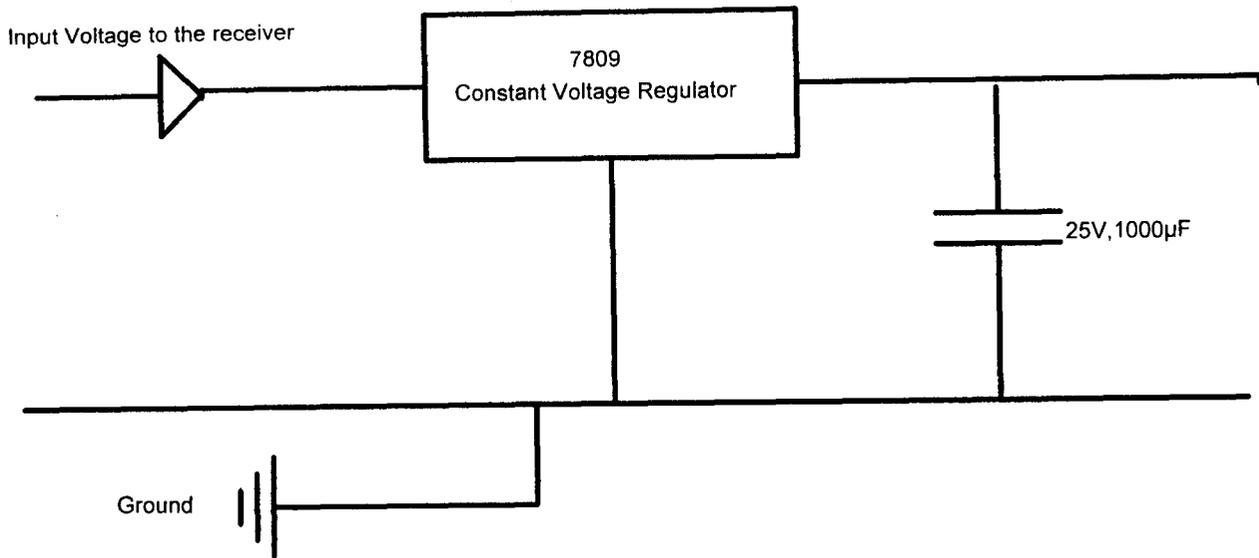
Fig.3.3 FM Receiver's power supply
