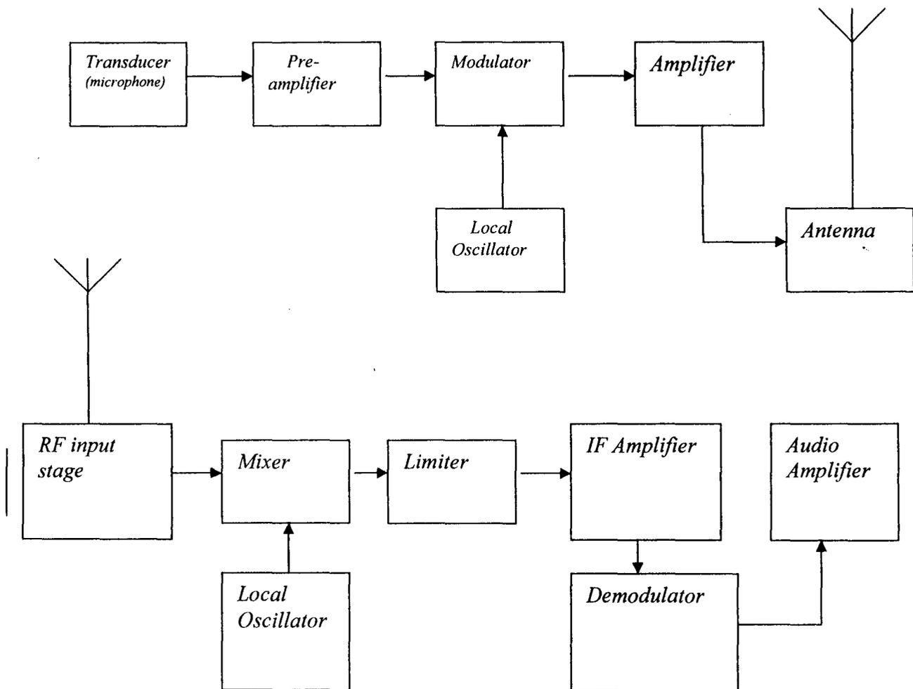
Fig 1.1 The block diagram of the wireless PA system.
