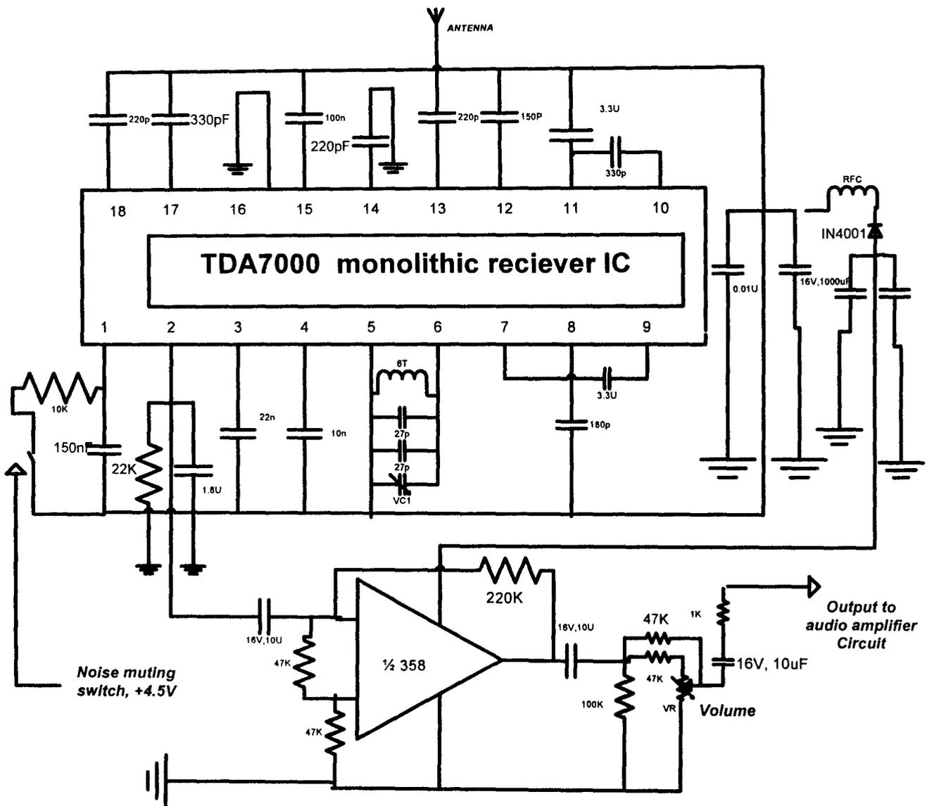
Fig.2.7 Circuit diagram of a TDA 7000 Frequency Modulation Receiver (all ground connection should terminate at pin 16)
