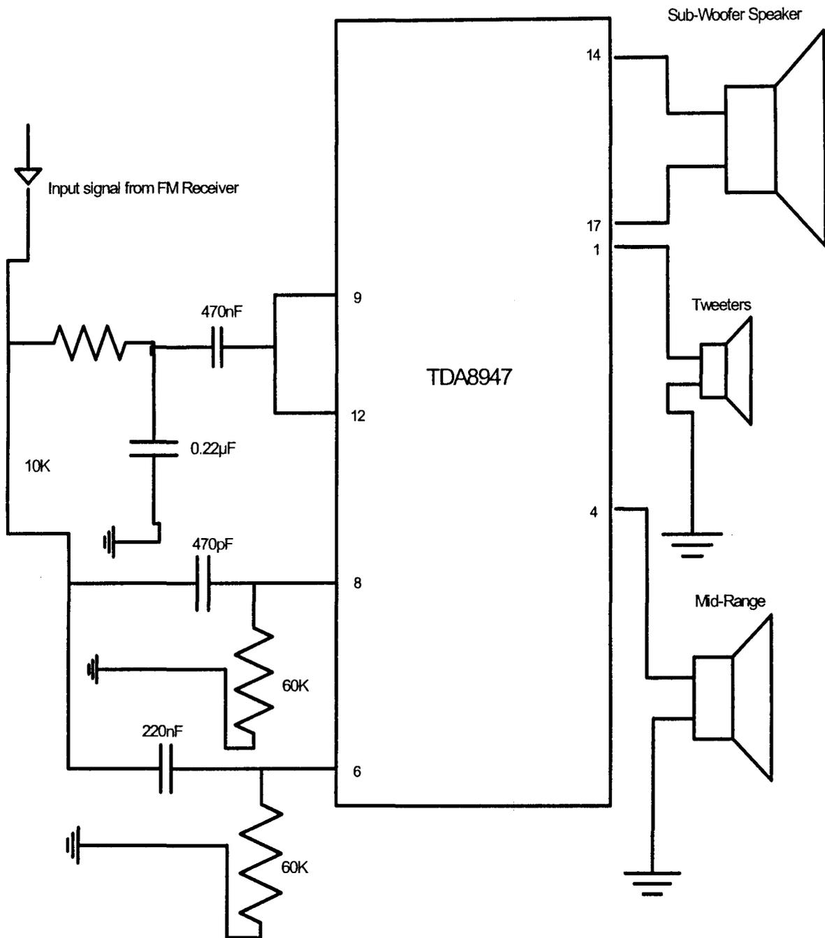
Fig. 3.6 Pin connection of the Power Amplifier to the loud speakers
