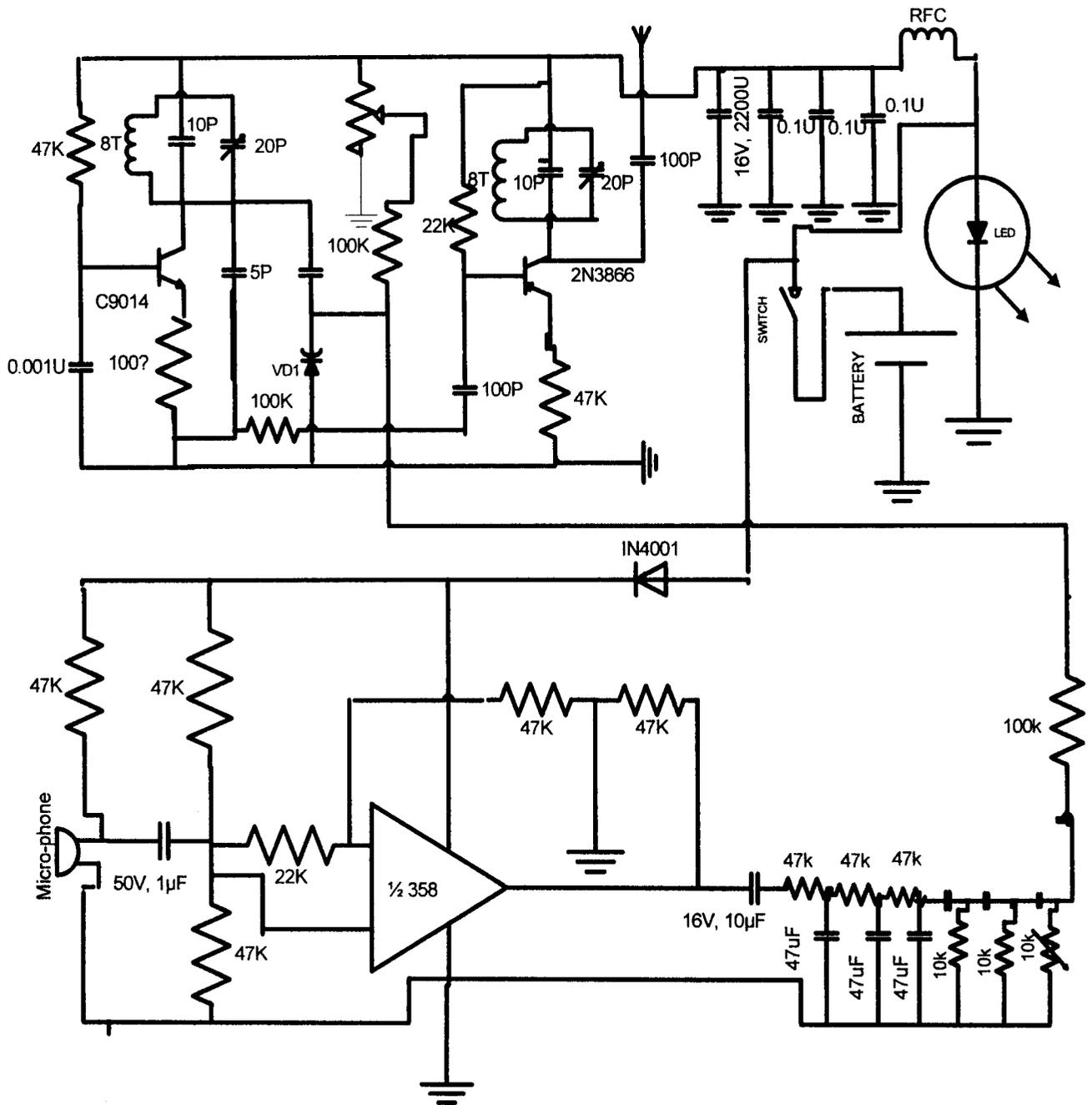
Fig. 3.4 A varactor Diode FM transmission circuit
