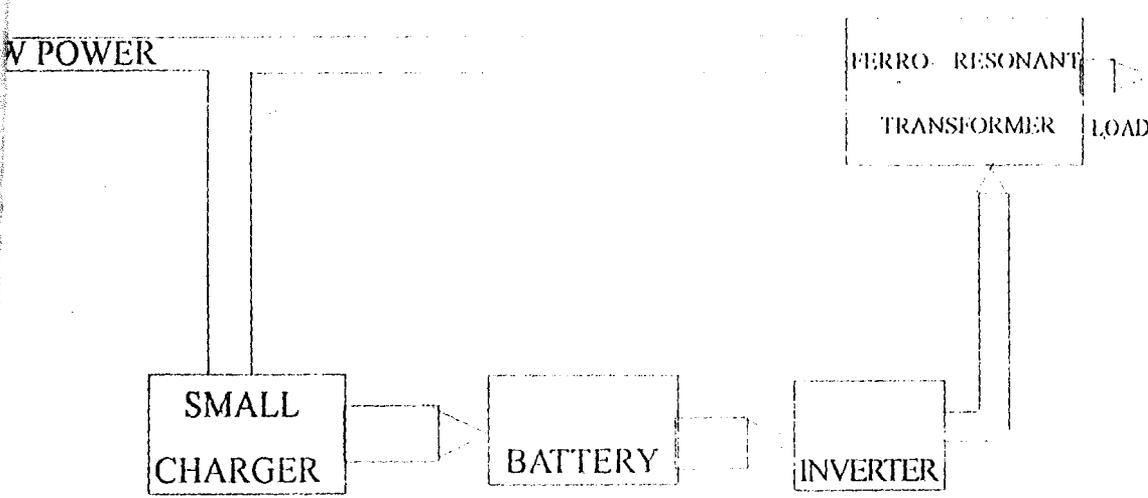
Fig 1.4 FERRO RESONANT UPS
