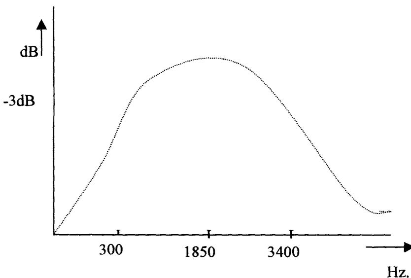
Fig. 2.2 (B) Frequency response of the band – pass filter.
