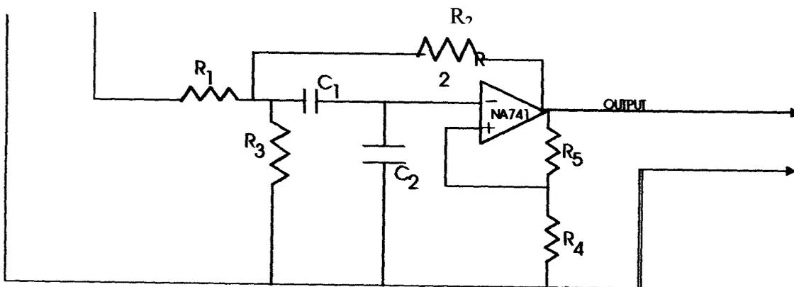
Figure 2.2(a) Band pass filter circuit.
