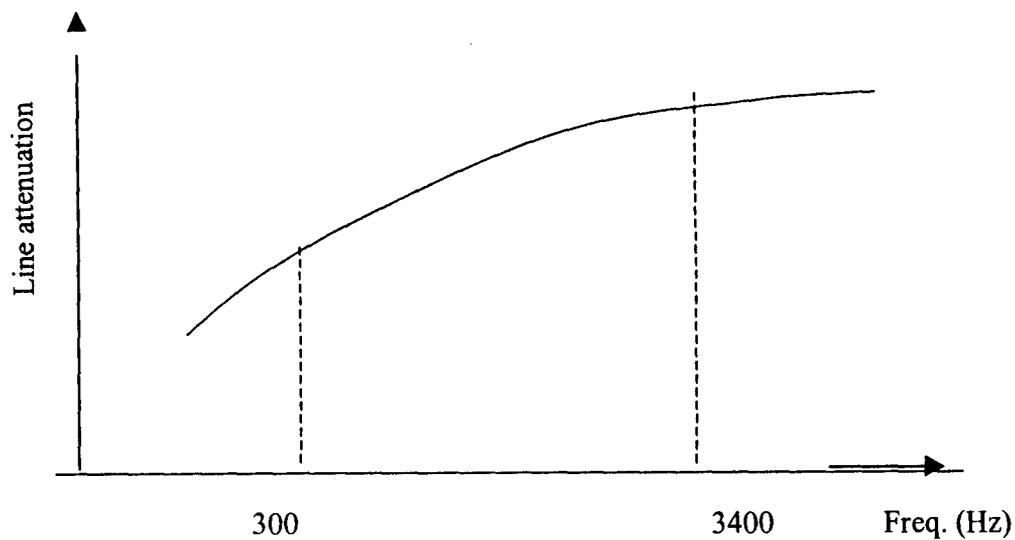
Fig.2.2(a) Attenuation Frequency characteristics.
