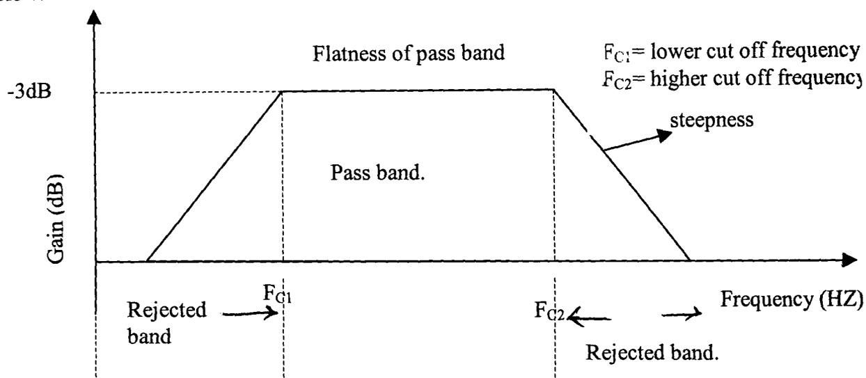
Fig. 2.2(b) Frequency Response of a band pass Filter.
