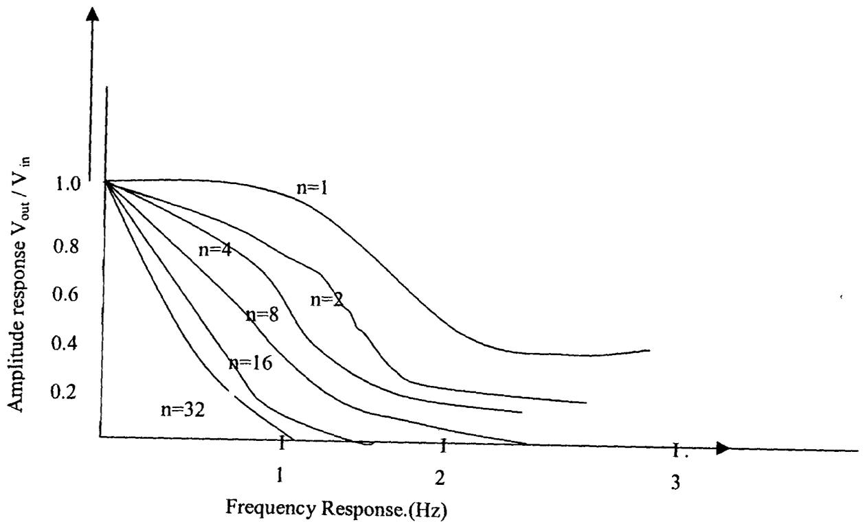
Fig 2.2 (b) Frequency response of multi section RC filters.
