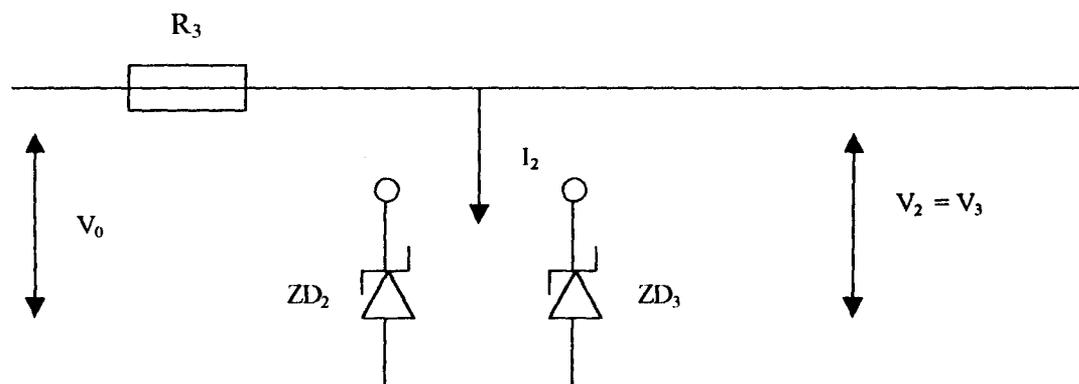
**Fig 2.1 (e) Shunt regulator- (voltage).**
