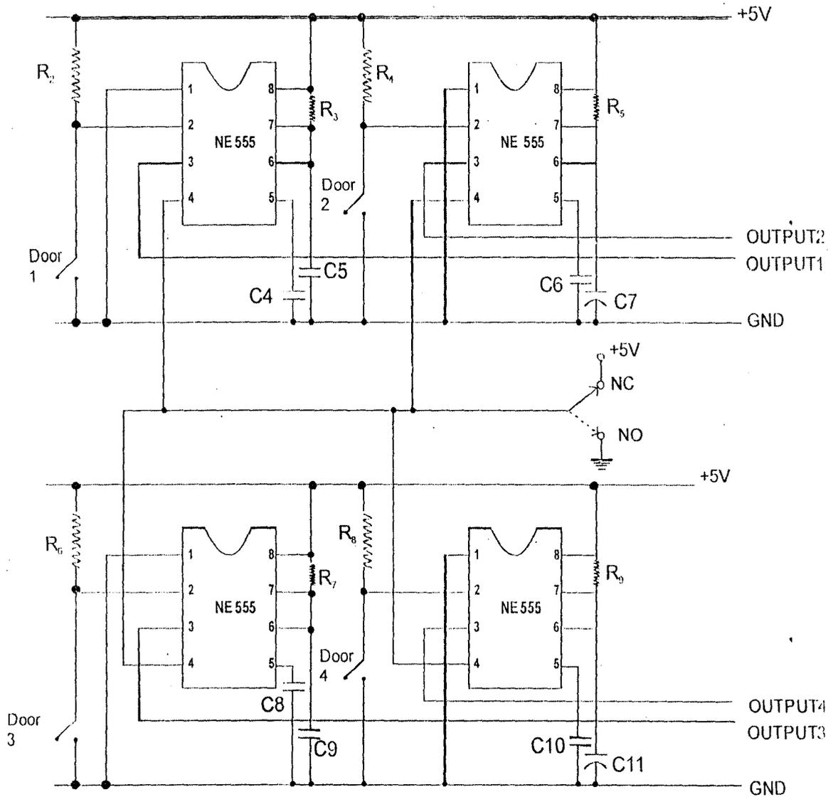
Fig. 3.4 Circuit Diagram of the trigger unit
