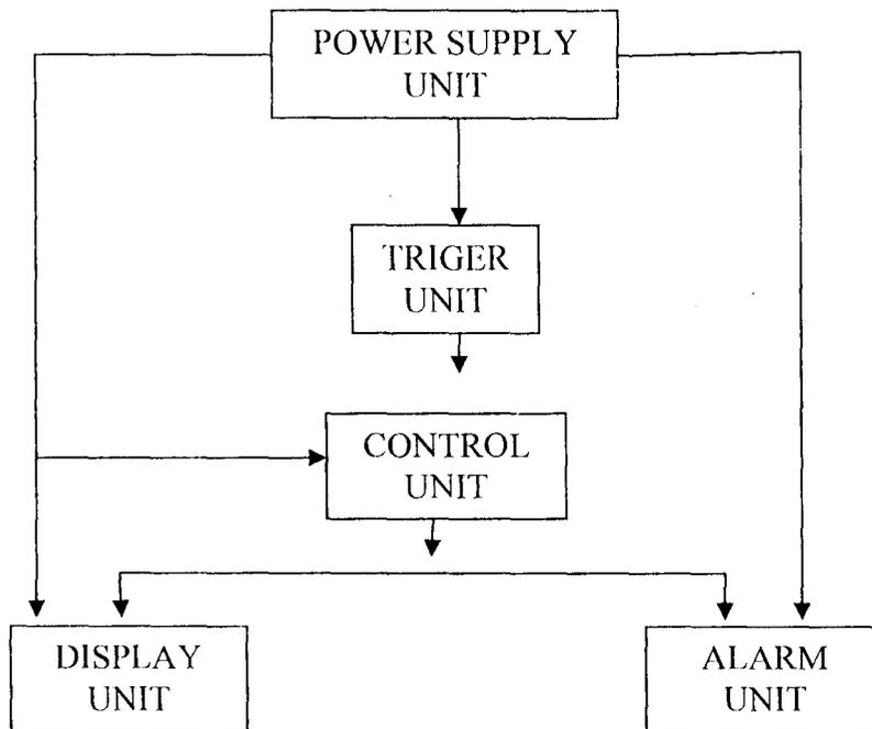
Fig. 3.1 Block diagram of four-door monitoring alarm system
