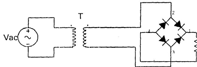
Fig 2.3d Complete Circuit Diagram of a Full Wave Bridge Rectifier
