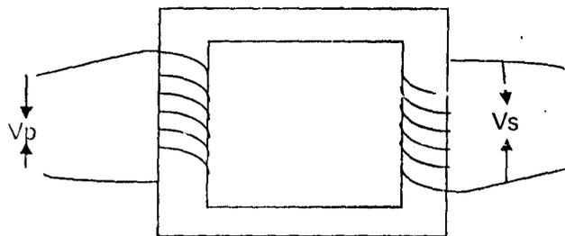
Fig 2.2 Diagram of a Transformer
