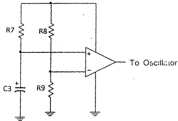
Fig. 3.5 Time delay Circuit
