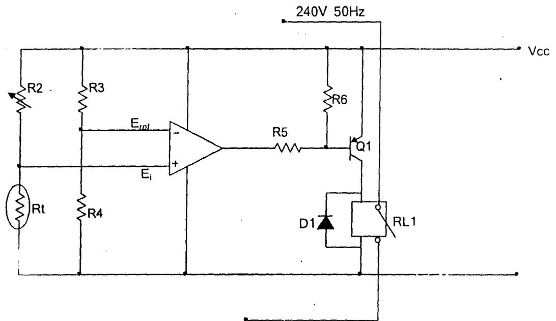
Figure 3.3 temperature control circuit
