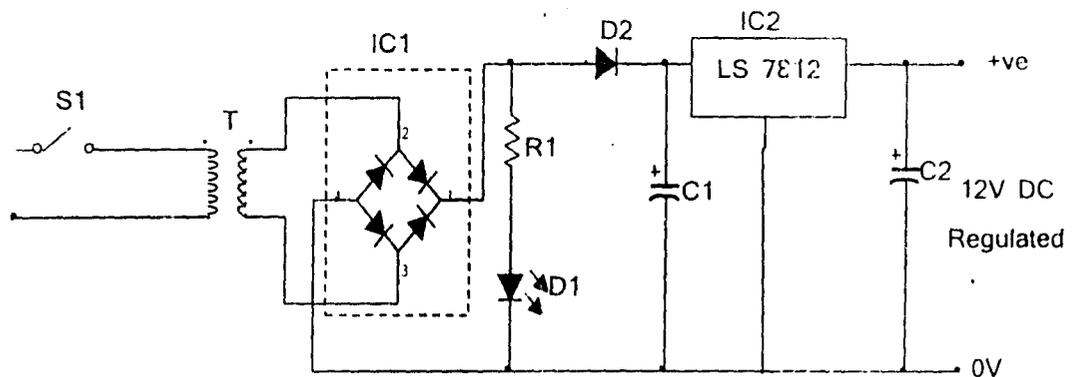
fig 3.2: 12v dc regulated power supply circuit design
