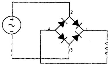
Fig 2.3c Full Wave Bridge Rectifier
