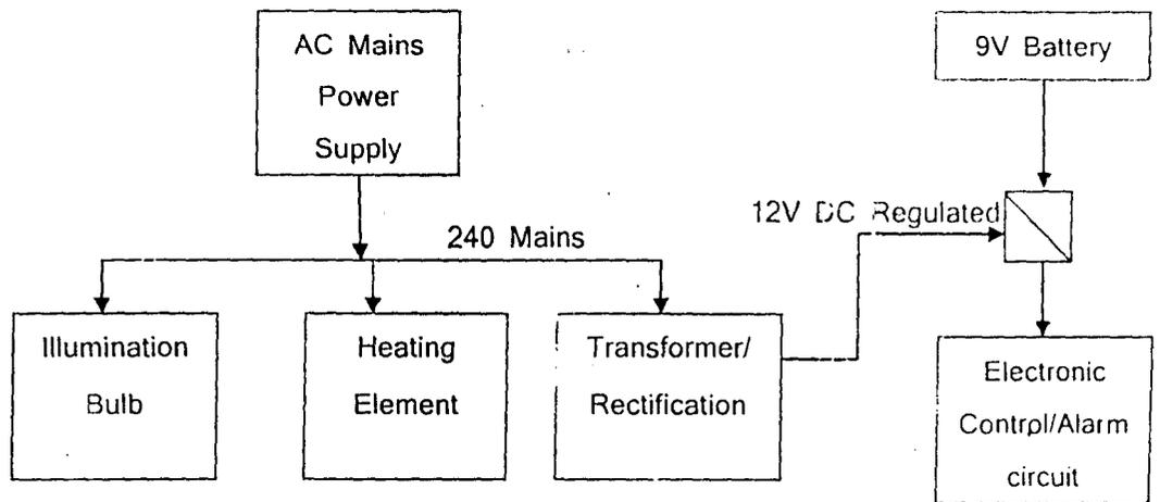
Fig 3.1 block diagram of power supply distribution in incubator
