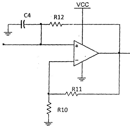
Fig. 3.6 Oscillator Circuit
