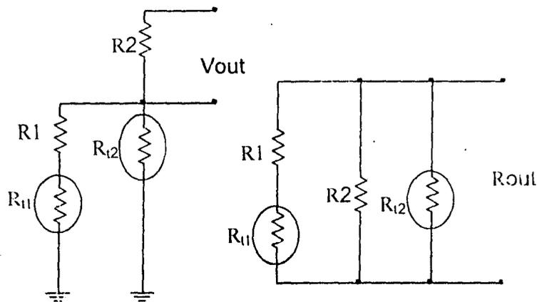
Fig 2.6 Circuit Diagram of a Transducer
