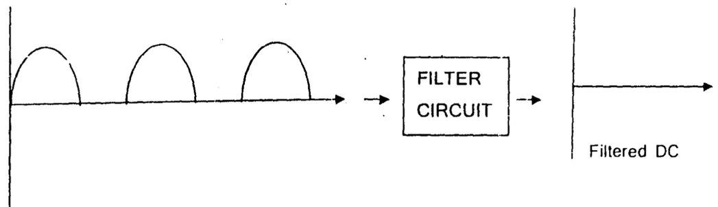
Fig. 2.4 Diagram of a Filter Function
