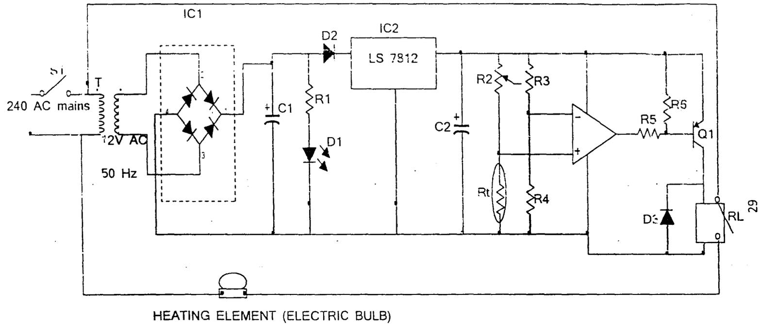
Fig. 3.7 COMPLETE CIRCUIT DIAGRAM OF AN EGG INCUBATOR
