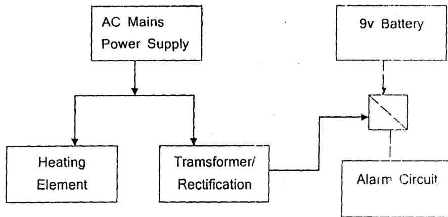
Figure 2.5: block diagram of power distribution in incubator
