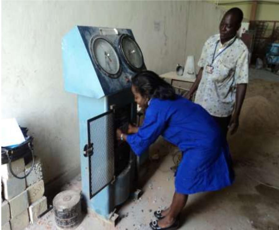
Taking reading of the crushing load
