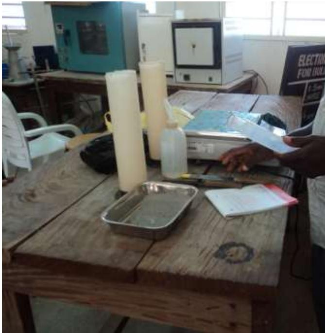
Doing the specific gravity test for the materials used.
