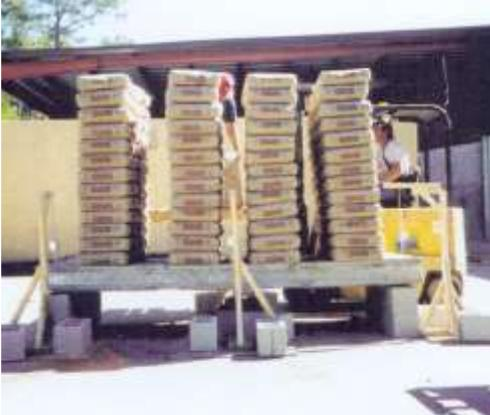
An EPS slab being tested via axial loading in Mborá district.
