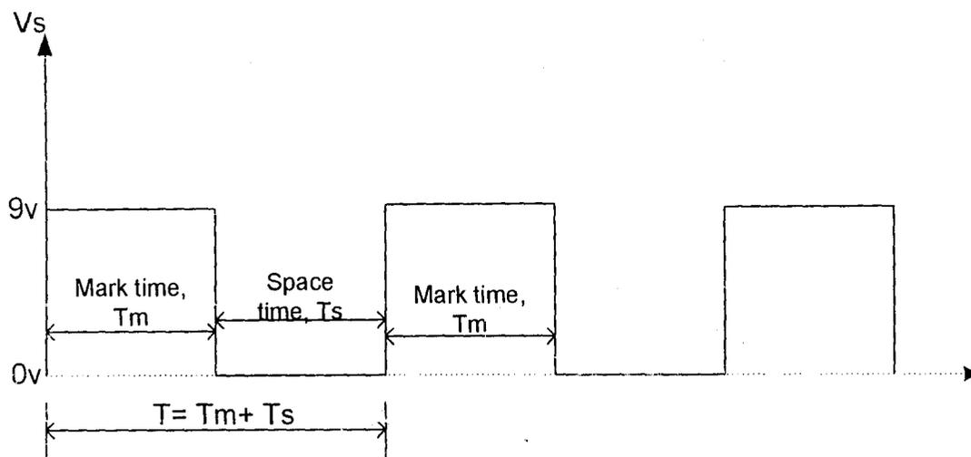
FIG 4. 1b Graphical Representation of the Siren Output
