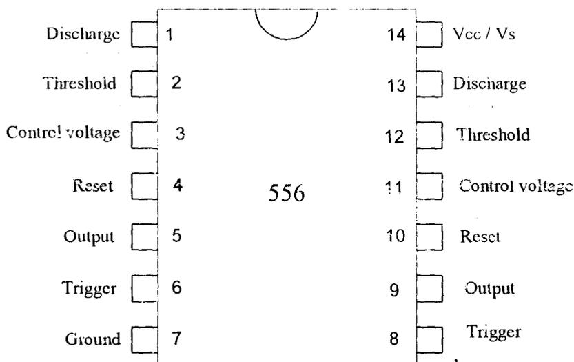
FIG 3.2 Pin Configuration of the 556 Integrated Circuit (IC)
