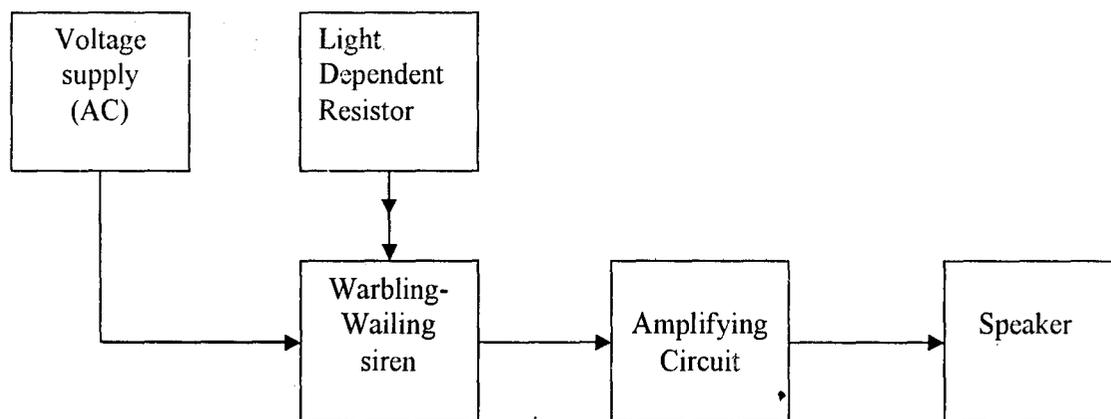
FIG 1.1 Block diagram of warbling-wailing siren with light dependent resistor
