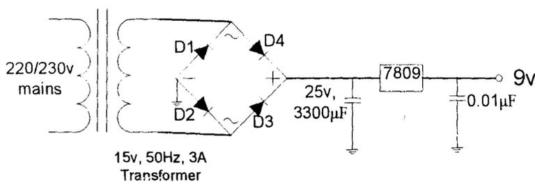
FIG 3.0 Power Rectification Process to 9v
