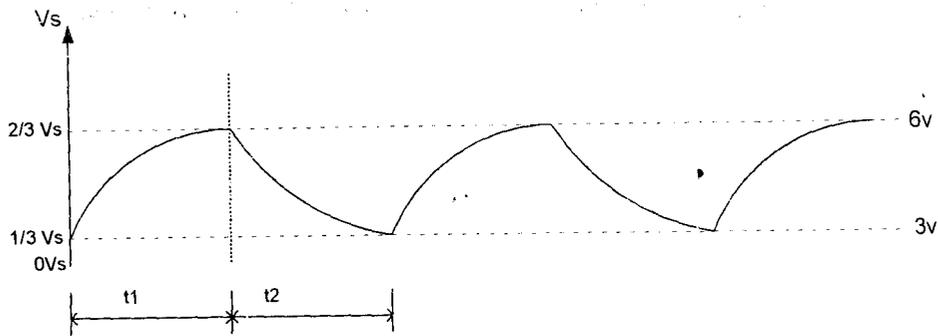
FIG 4. 1a Graphical Representation of the Capacitance Variation.
