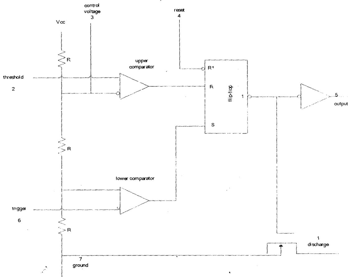
FIG 3.3 General Functional Block Diagram Of The 556 In Astable Mode
