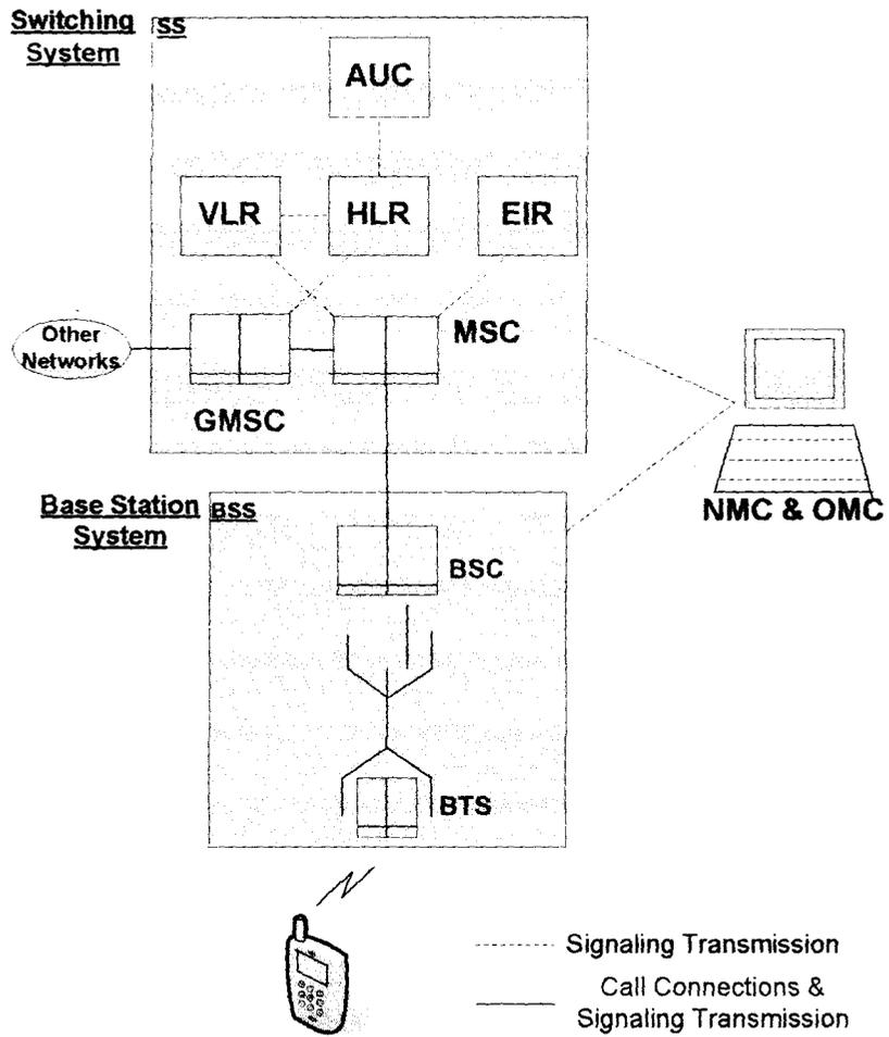
**Figure 2.3.1: GSM Network Component**
