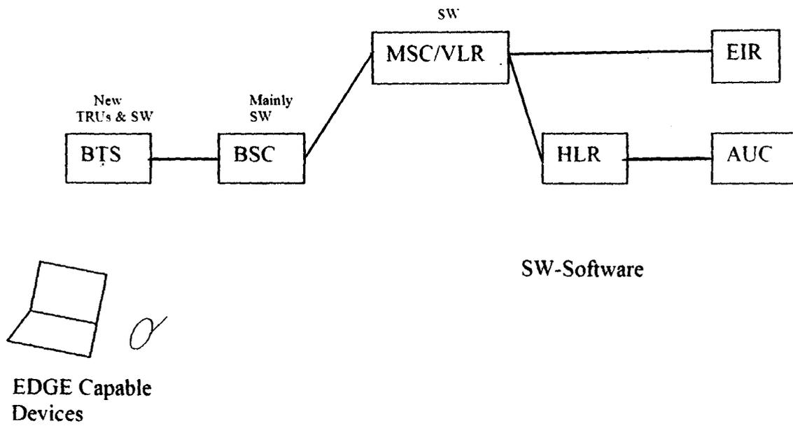
**Figure 5.4.4: Diagrammatic Representation of the Network Modification Due to EDGE (3G)**
